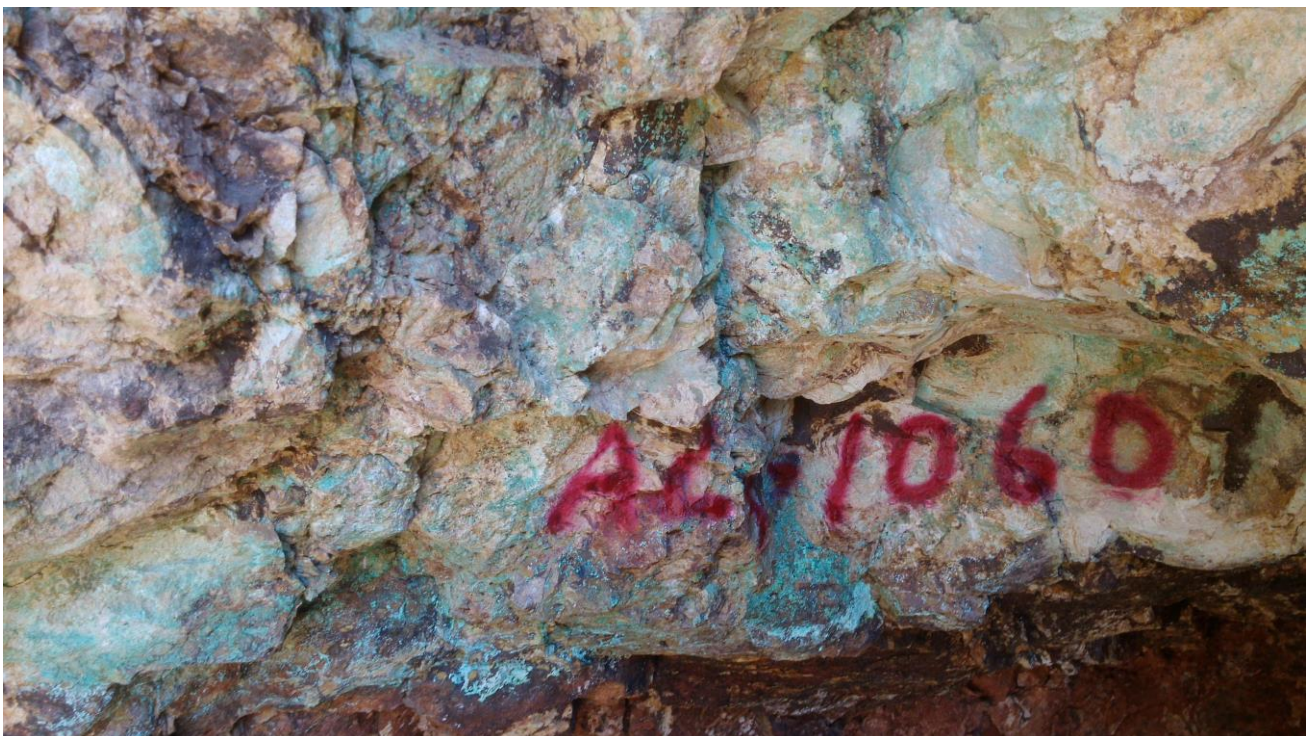
Photo 1: Copper oxide mineralisation in La Morita mine workings: a 1.8m channel sample (ALR-1060) across the back returned a grade of 5.36% Cu
