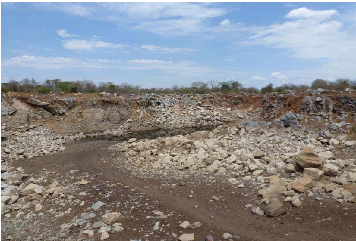
Figure 2: Industrial minerals geologist Robert Barnett at site. Figure 3 this quarry has been mined to 10 metres depth for road base – sampling shows it contains cement grade limestone and that the mineralisation is open in all directions.
