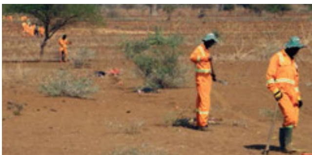
Photo 4: Layout crew positioning geophones during the Moshi survey
