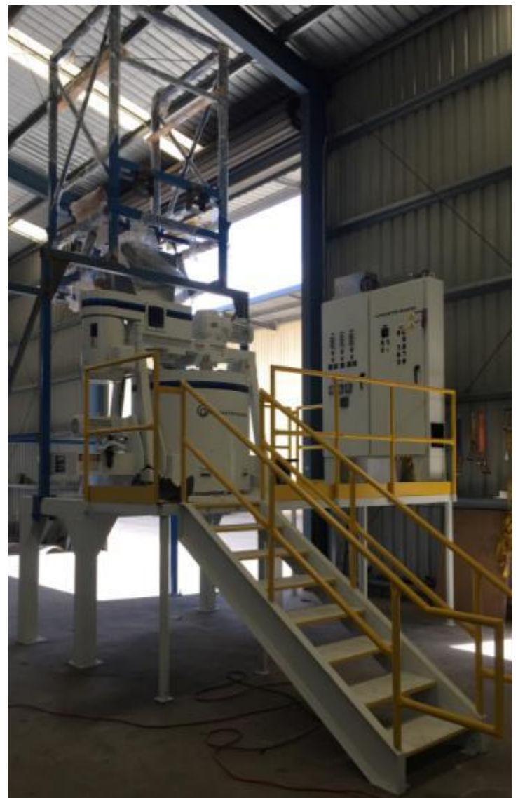
Image 2: Granulator installation completed, awaiting commissioning.
