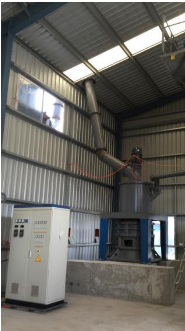
Image 1: Fine Grinding Mill complete, commissioning completed.
