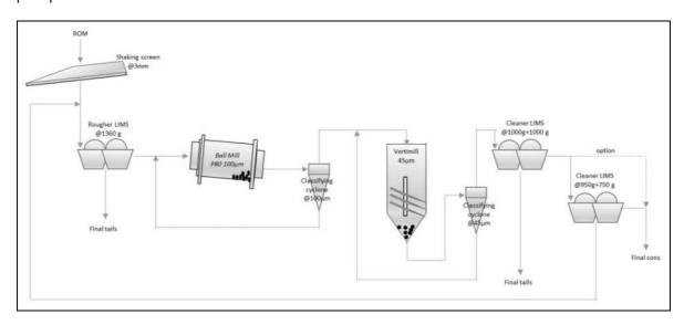
After significant test work carried out by MBE labs in Germany and CRL in New Zealand, a process flow diagram ('PFD') has been agreed by all parties. This PFD is based on a 1 stage rougher magnetic separator (LIMS is acronym for Lower Intensity Magnetic Separators), followed by a 3 stage lower gauss 'cleaner' magnetic separators. To grind the raw material to an optimal level of magnetic iron liberalisation, a ball mill and vertimill configuration is utilised to achieve a 45 micron sizing.
