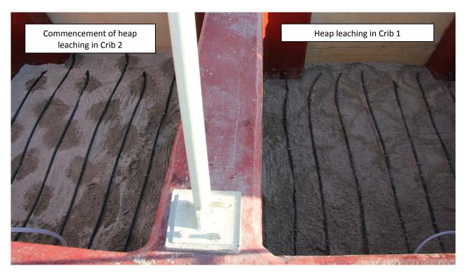
Commissioning of the plant is well underway and by late April three of the cribs were loaded with 40 tonne samples and drip feed acid leaching commenced. Bannerman remains on track to deliver first test results in the June quarter 2015.
