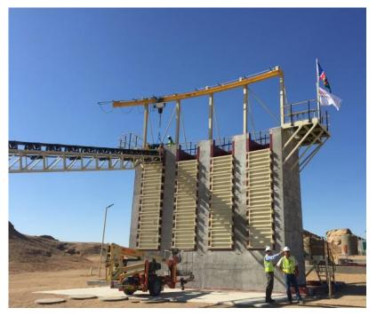
The four 2m x 2m x 5m cribs enables heap leaching of individual 40 tonne samples as well as simulating the planned heap leach pad operation through circulating the leached solution between the cribs.
