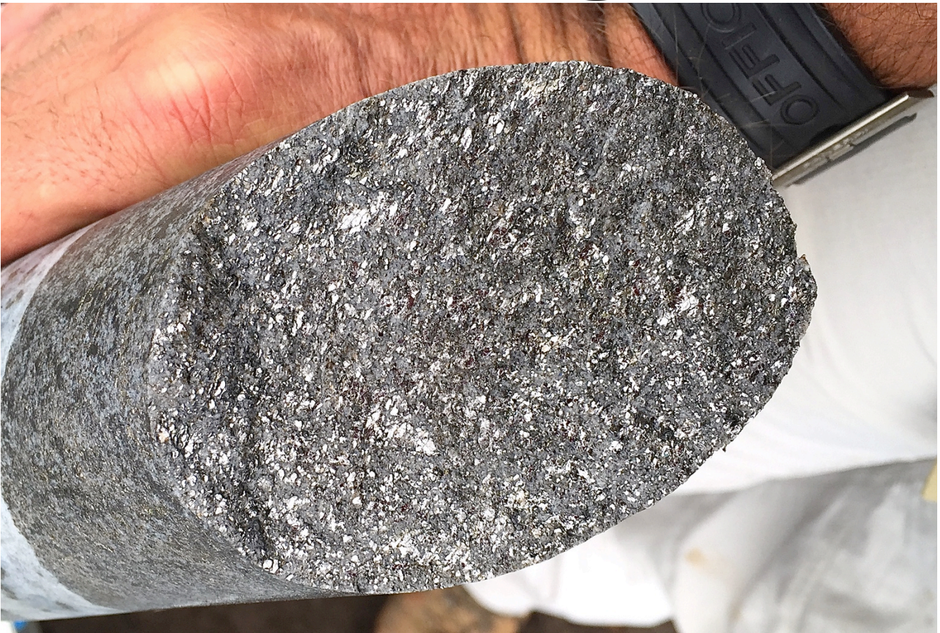
Photo of diamond core at DD01 showing coarse graphite flakes 0.5–2.0mm. Core diameter is 64mm
