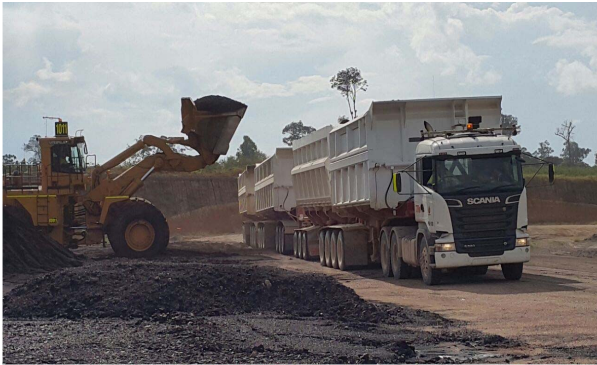
Photo 1 – New Scania haulage trucks (300 tonne capacity) transporting coal from BAYAN’s existing TABANG mining concessions to Senyur Port using the new 69Km long coal haul road.
