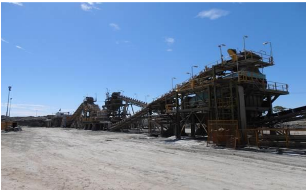
Figure 1: SIGM heap leach 3 stage crushing and screening plant (courtesy SIGM)
