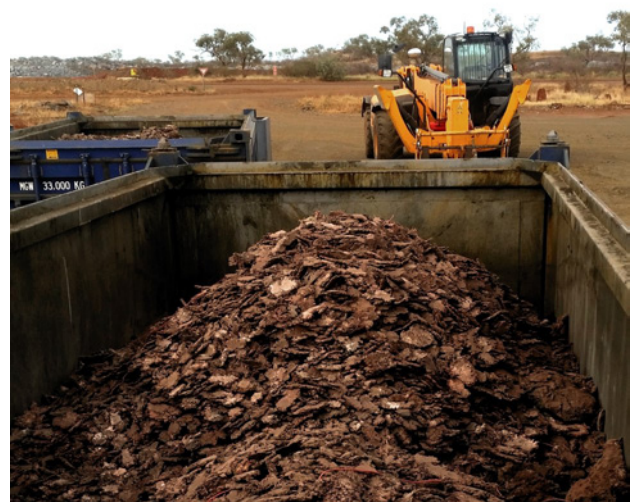
Figure 20: Ore sorter circuit is producing high-grade coarse native copper product ranging from 85-95% Cu metal in concentrate. The oversize native copper nuggets that are too large for the main mineral processing plant (designed for -40mm fraction), are being removed, in the process generating a valuable additional copper concentrate product.
