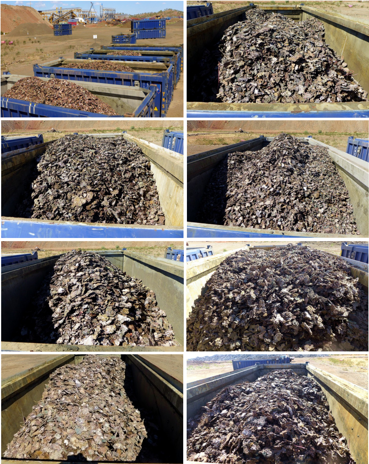
Figure 19: Coarse native copper product ranging in grade from 85-95% copper metal in concentrate. The purpose of this circuit is to remove oversize native copper (+40mm) prior to commencement of processing in main mineral processing plant under construction.
