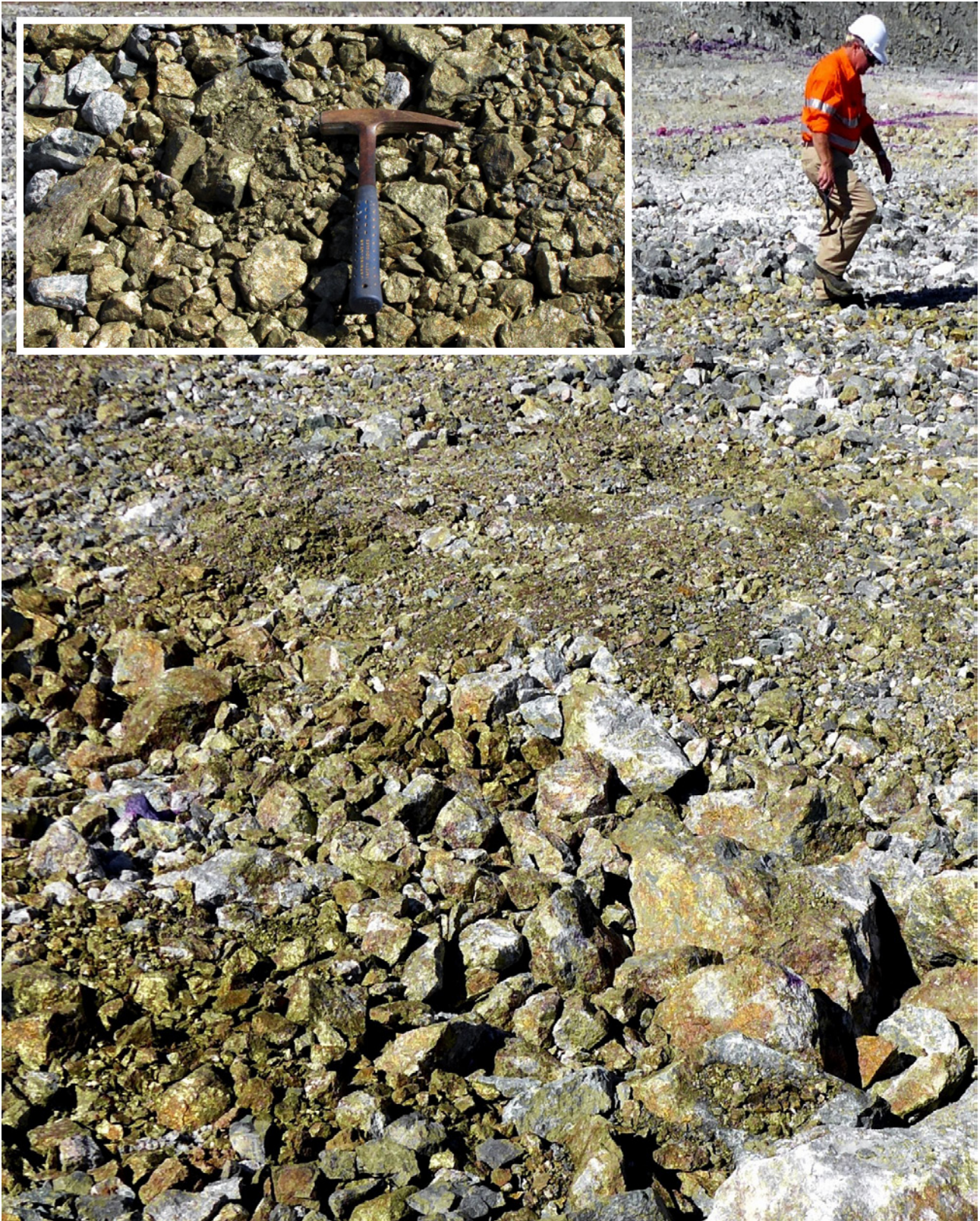
Figure 14: LM2 Pit floor at RL195 - high-grade primary copper ore (chalcopyrite) including massive, semi-massive, breccia, fracture infill, and disseminated, strewn across the pit floor.
