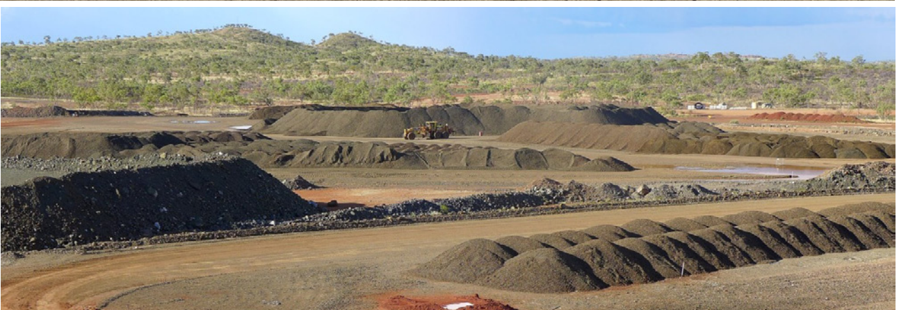
Figure 21: Ore sorter circuit is producing high-grade coarse native copper product ranging from 85-95% Cu concentrate. Bottom image shows crushed native copper ore stockpiles ready for processing. Rocklands native copper metal contains 99.65%Cu.
