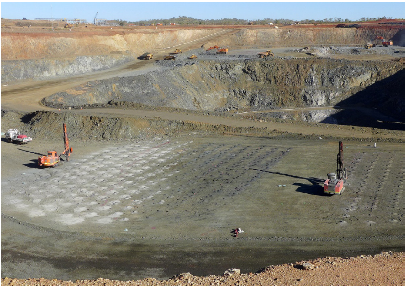
Figure 12: Top image shows the south end of the LM2 Pit where high-grade primary copper sulphide ore (chalcopyrite) is being mined. Bottom image shows blast-hole drilling at the north-end of the LM2 Pit - the highly weathered supergene ore stands out against the lighter coloured adjacent fresh rock.
