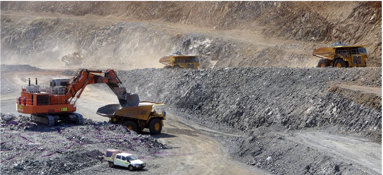
Figure 16: LM2 Pit floor at RL195 - approximately 60m wide ore zone of very high-grade primary copper ore (chalcopyrite, bornite, chalcocite), cobalt ore (pyrite) and magnetite, strewn across the pit floor.
