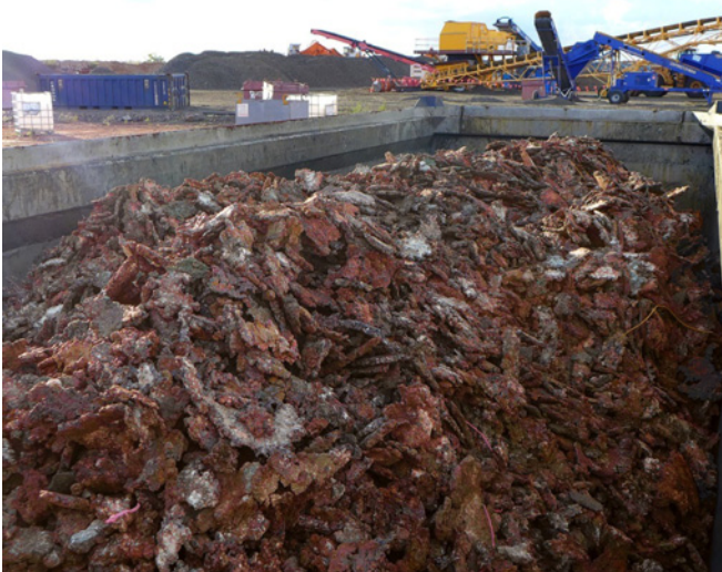
Figure 20: Ore sorter circuit is producing high-grade coarse native copper product ranging from 85-95% Cu metal in concentrate. The oversize native copper nuggets that are too large for the main mineral processing plant (designed for -40mm fraction), are being removed, in the process generating a valuable additional copper concentrate product.
