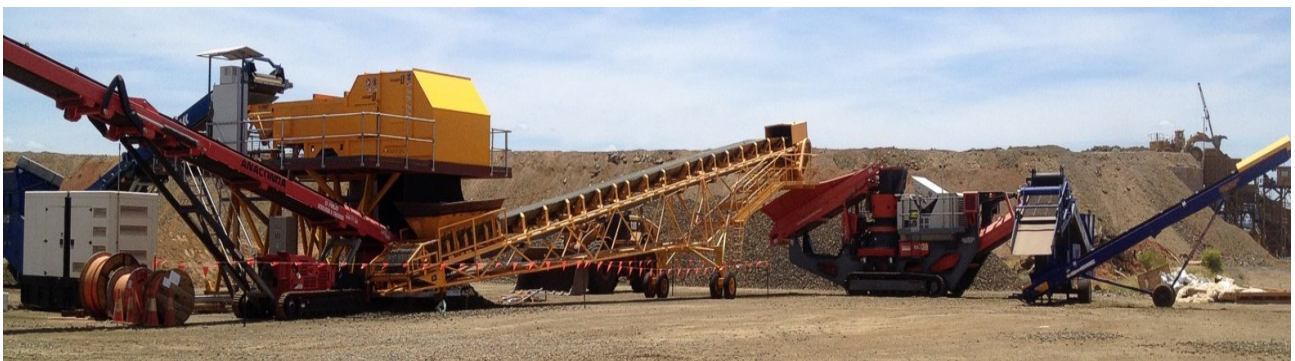
Figure 18: Ore sorter circuit is producing high-grade coarse native copper product ranging from 85-95% Cu metal in concentrate.
