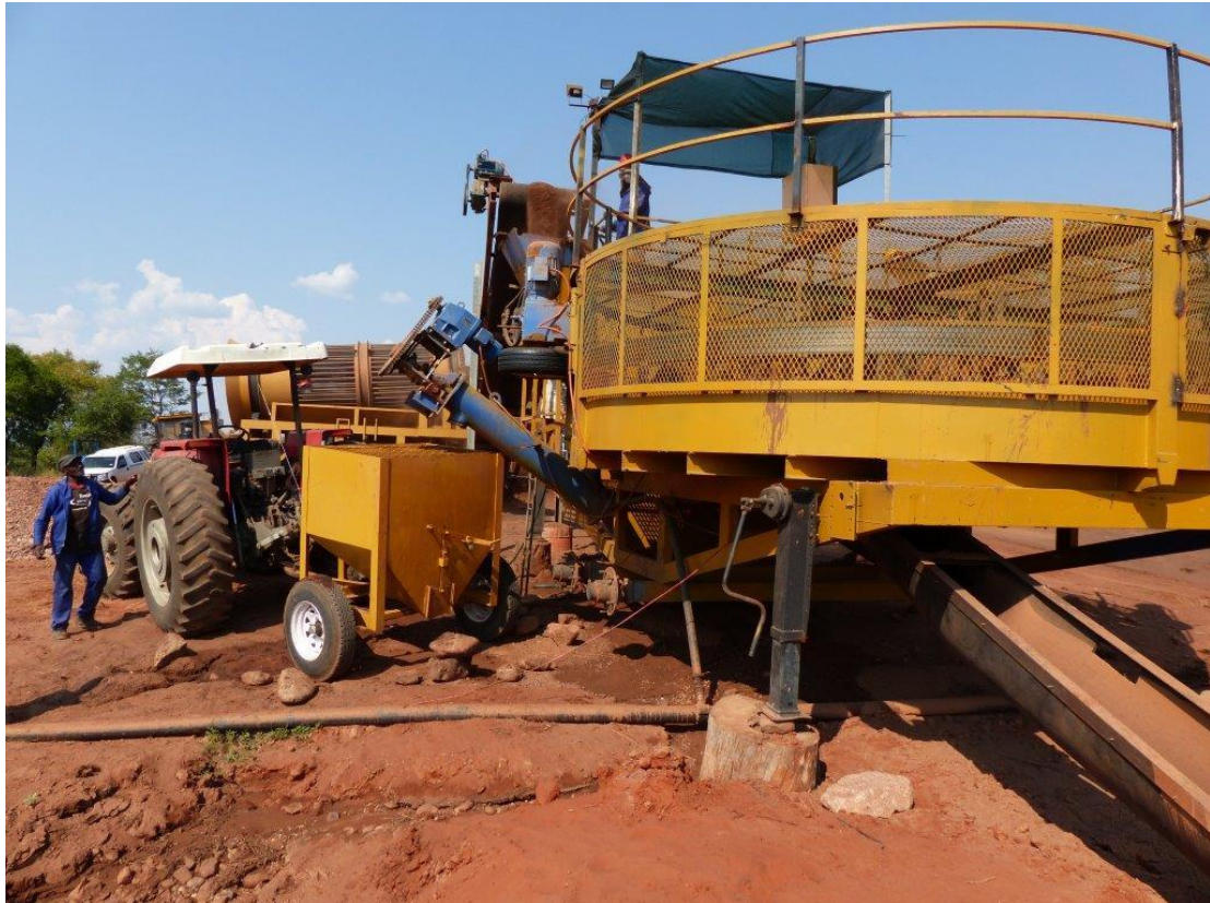
16-foot rotary-pan used for concentrating heavier minerals (incl. diamonds)
