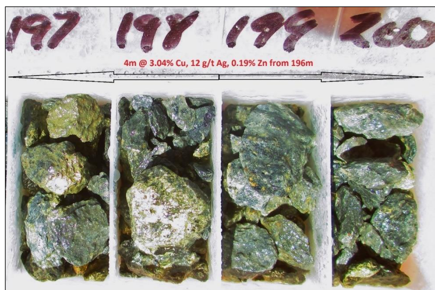
Figure 4 – WLRC005 RC drill chips showing chalcopyrite mineralisation within sheared felsic volcanic
