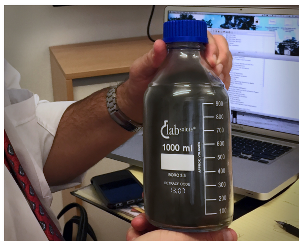
Fig 2. Graphene powder produced by Dresden University of Technology from Vittangi drill core.
