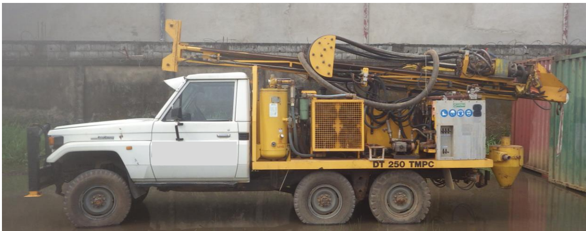
Figure 1: Aircore drilling rig mounted on a six wheel drive Toyota Landcruiser acquired by Canyon
