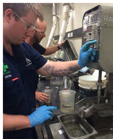
Figure 4. Flotation testwork being conducted at ALS Laboratory
