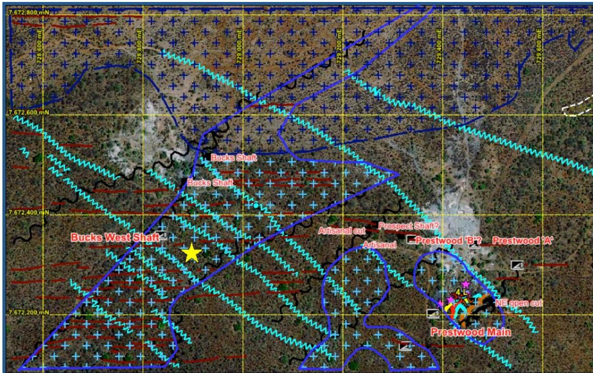
The above images shows the position of newly developed artisanal shafts (Yellow Star), superimposed on Quick Bird Imagery . The structure hosting the mineralisation parallels the one that hosts the old Bucks West (and West ventilation) shafts and Prestwood Shafts, 430m to east. Interpreted monzonite sub outcrop is shown as blue crosses. SW-NE shears as black wavy lines, and SE-NW cross shears as light blue wavy lines.
