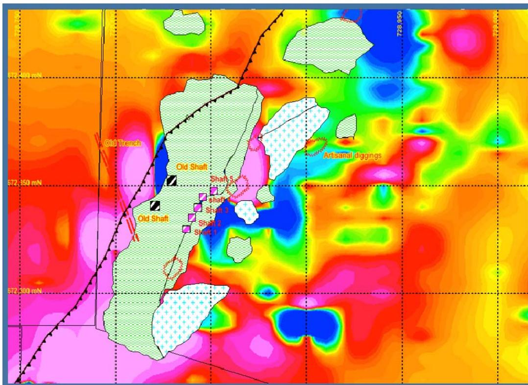
*The above image shows the position of newly developed artisanal shafts on SW – NE structure, superimposed on total magnetics. This structure parallels the one that hosts the old Bucks West and West ventilation shafts. Greenstone outcrops are indicated in light green, with monzonite with blue crosses.*
