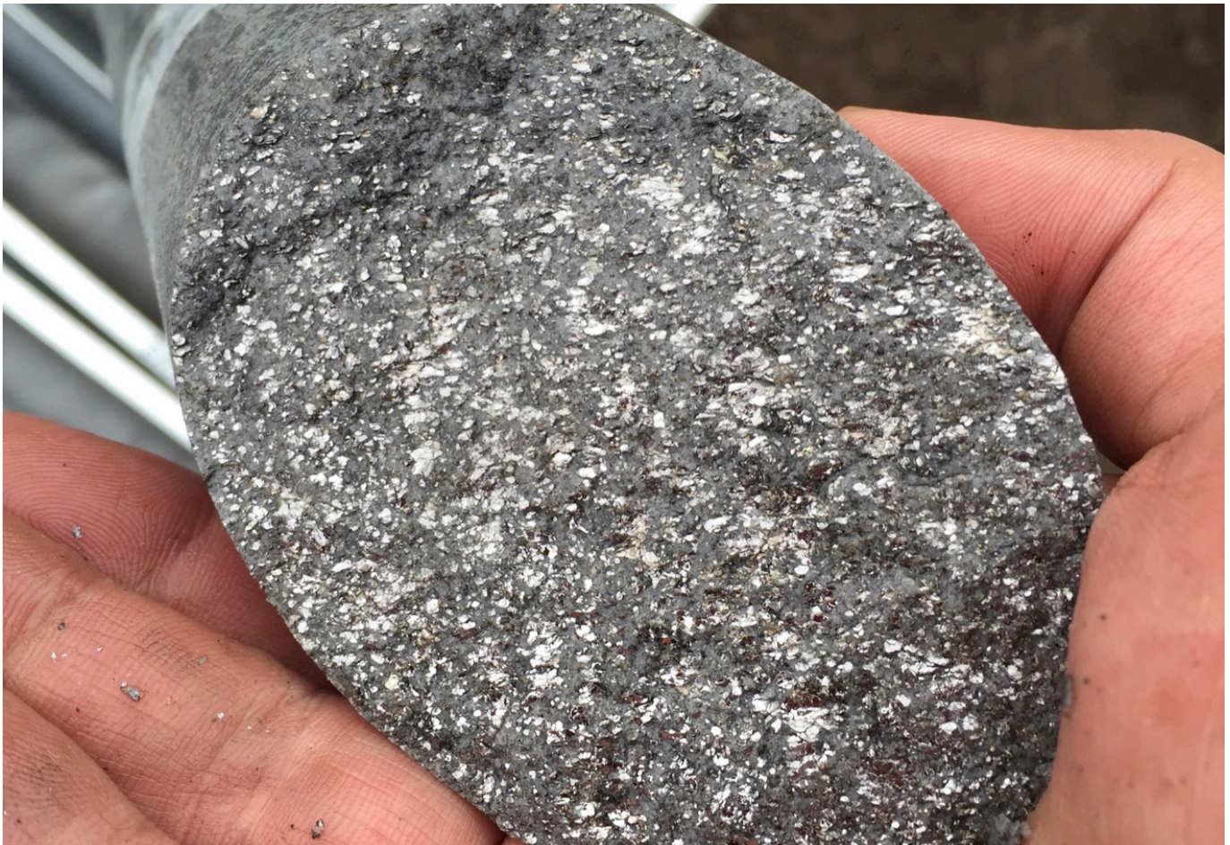
Photo 1. Coarse flake graphite seen in core sample from hole DD01 drilled in January this year. Core diameter is 64mm
