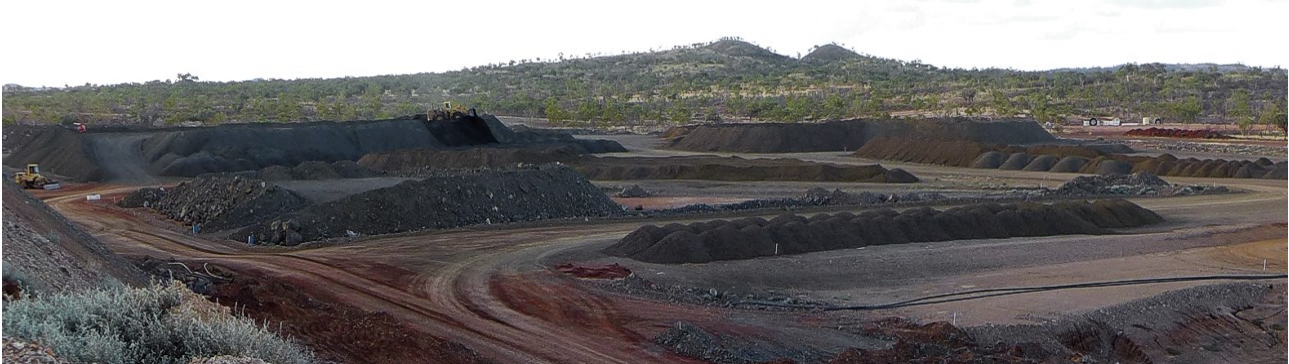
Figure 5: Crushed ore stockpiles (-40mm) will be fed directly into the Process Plant without further crushing, and are currently over 200,000 tonnes.
