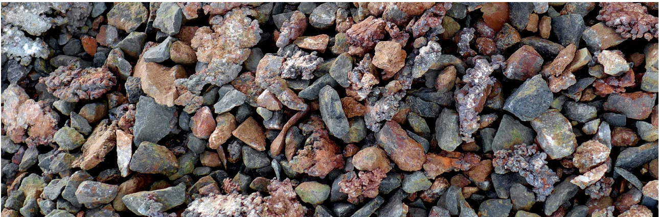
Figure 1: Close-up of high-grade crushed native copper ore (-40mm), after removal of coarse (+40mm) native copper
