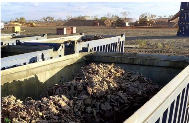
Figure 3: The native copper scalping programme is generating an extremely high-grade native copper metal product (~95% copper) for interim sales and early cash-flow. This shipment is due for export in May to Chinese smelters. Once the coarse native copper metal has been scalped, the remaining crushed ore (<40mm) is stockpiled for future direct feed to the Process Plant, avoiding re-crushing and resulting in future cost savings.
