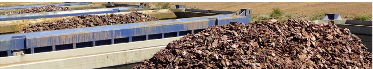
Figure 2: Oversize native copper metal concentrate ~95% Cu loaded into containers at Rocklands prior to shipment to Townsville.
