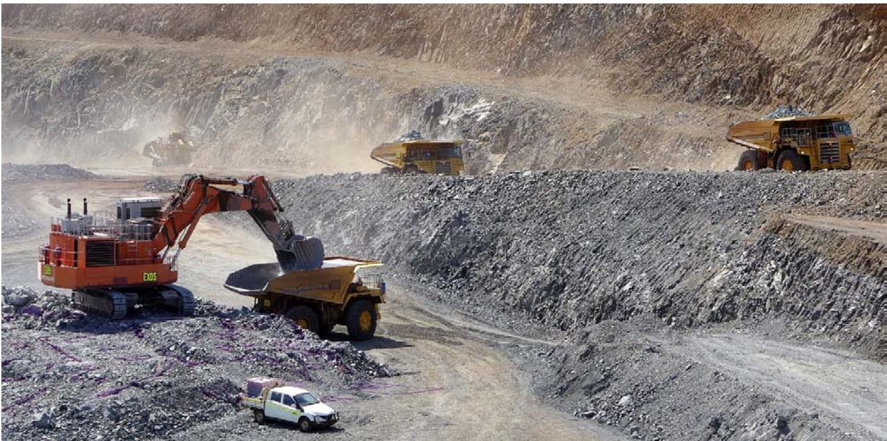
Figure 20: Mining primary ore in LM2 Pit at RL190 - ore mark-up can be seen on pit floor.
