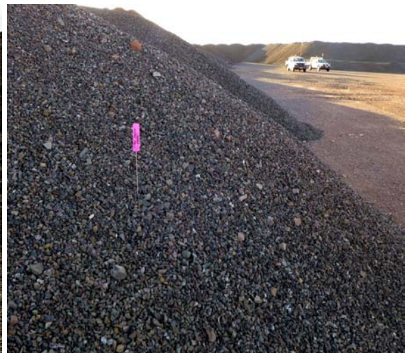
Figure 7: Crushed ore stockpiles (-40mm) grades are estimated from a combination of lab-assay of composite blast-hole samples and where not available, resource grade estimates are used. Check assays are regularly conducted for QAQC purposes.
