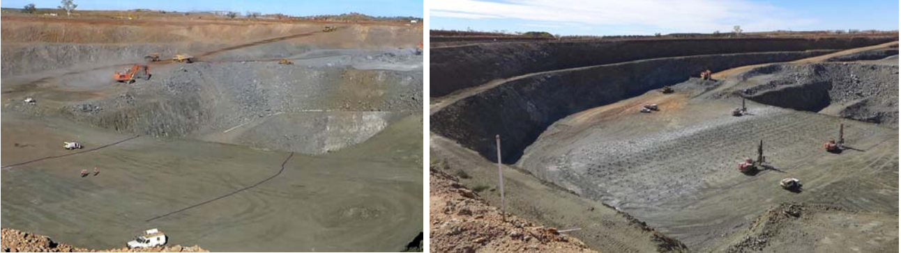
Figure 18: Blast-hole drilling the supergene ore at the north of LM2 Pit. Left image shows the ore-zone marked up (drilled first to expedite receipt of assays) , and the right image shows three blast-hole rigs concurrently drilling the ore zone.
