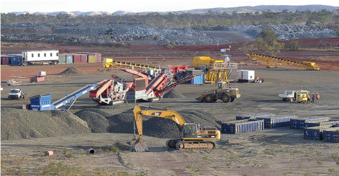
Figure 4: The native copper scalping programme is generating an extremely high-grade native copper metal product (~95% copper) for interim sales and early cash-flow. Once the coarse native copper metal has been scalped, the remaining crushed ore (-40mm) is stockpiled for future direct feed to the Process Plant, avoiding re-crushing and resulting in future cost savings.
