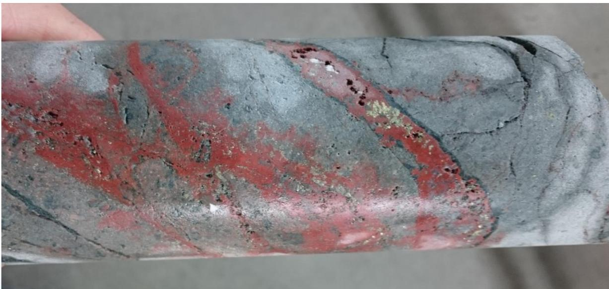
**Figure 3 – Drill core from NDD 001 at 81m showing albite alteration and pyrite-chalcopyrite in veins**
