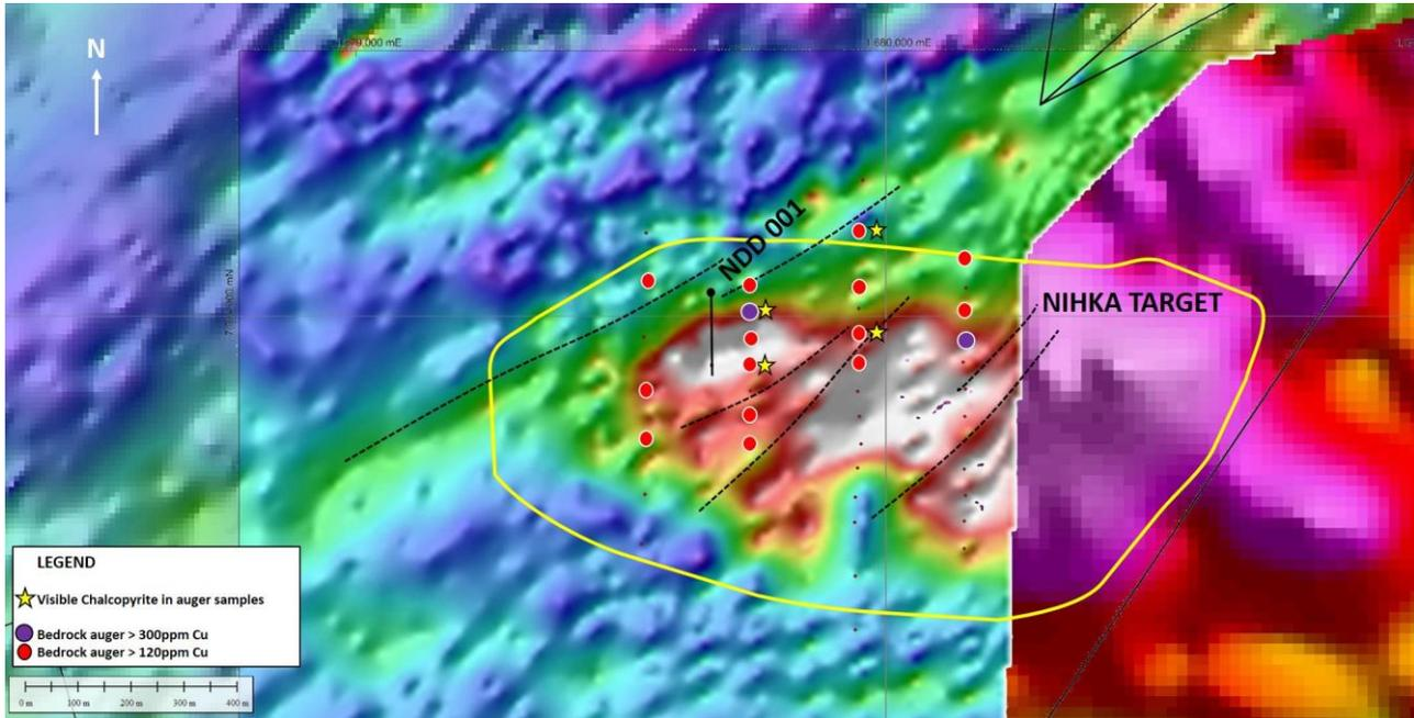
**Figure 2 –Location of drill hole NDD 001 at the Nihka target. The background image is ground magnetics (total magnetic intensity, SE shade). For the auger drilling results see announcement dated 9 April 2015.**
