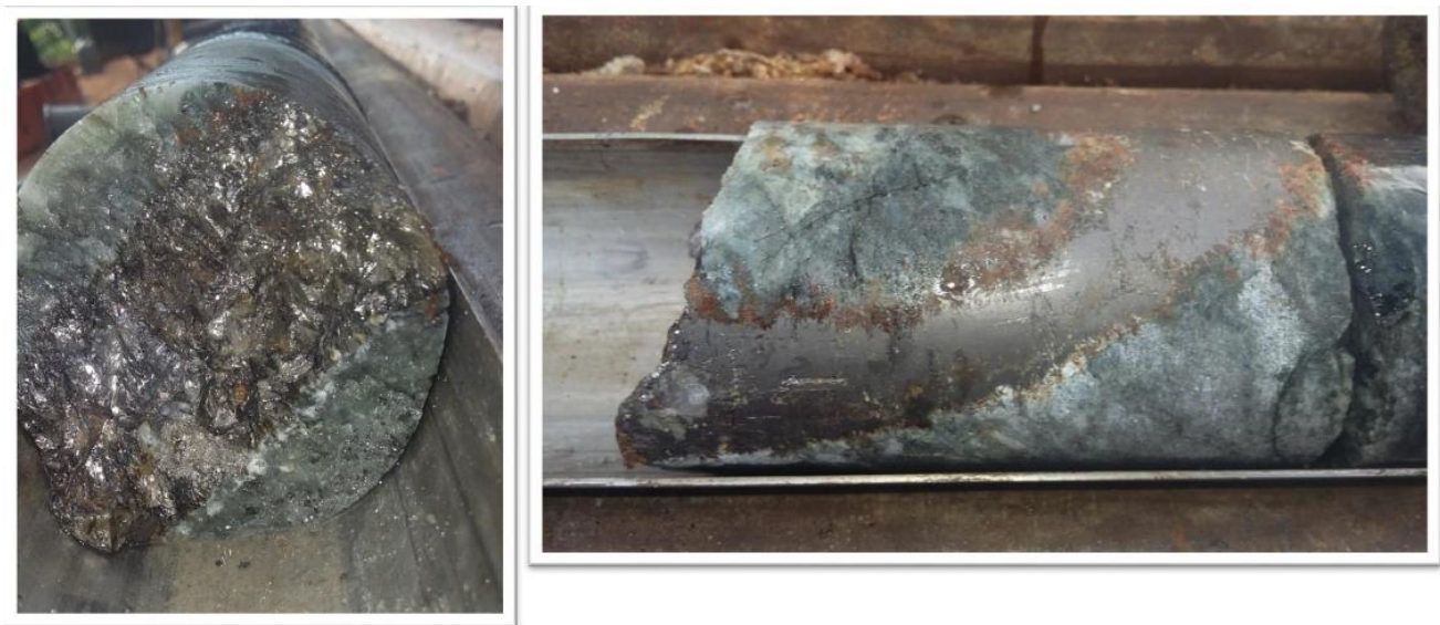
Figure 3 - Approximately 3-4 cm graphite vein @ 66.1m in PLB009
