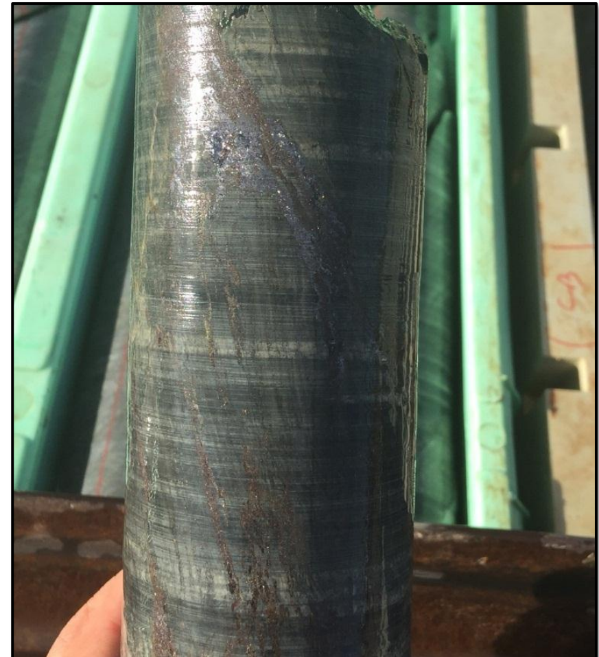
Drill core from HBRC001 approx 490m, showing intense chlorite alteration (khaki colour) with zinc sulphide (brown) and lead sulphide (silver) mineralisation.
