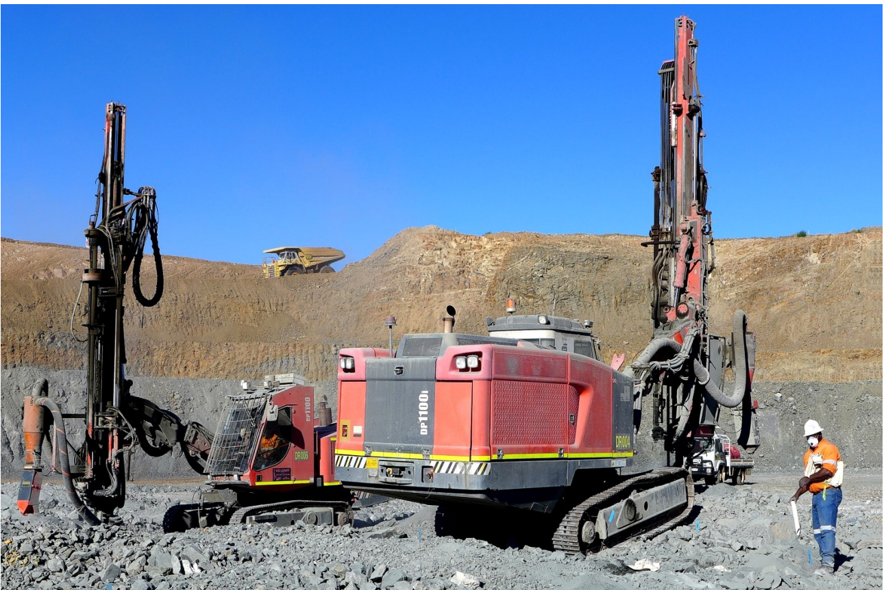
Figure 15: Blast-hole drilling in primary ore that is dominated by copper minerals chalcopyrite (34.6% Cu), with minor chalcocite (79.9% Cu) and bornite (63.3% Cu), at the south end of the LM2 Pit. Blast-hole returns are sampled in 5m composites by geologists or senior pit technicians, and sent for analysis at independent laboratories.
