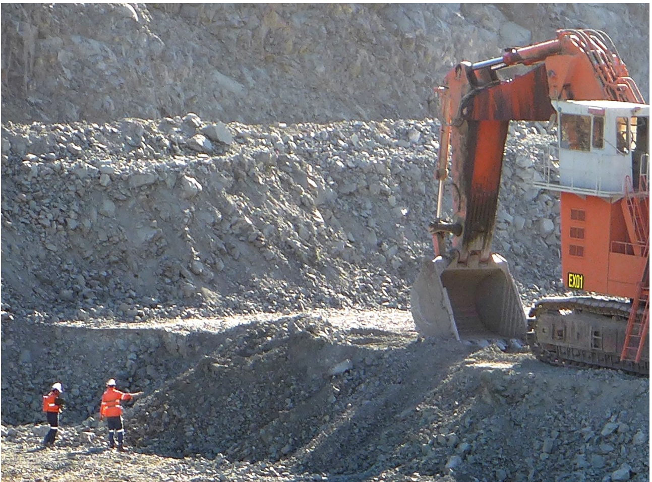
Figure 16: Ore control is based on pre-determined dig-plans projected onto the pit floor (top image), however grade control geologists also monitor every bucket of ore that is loaded into the dump trucks.
