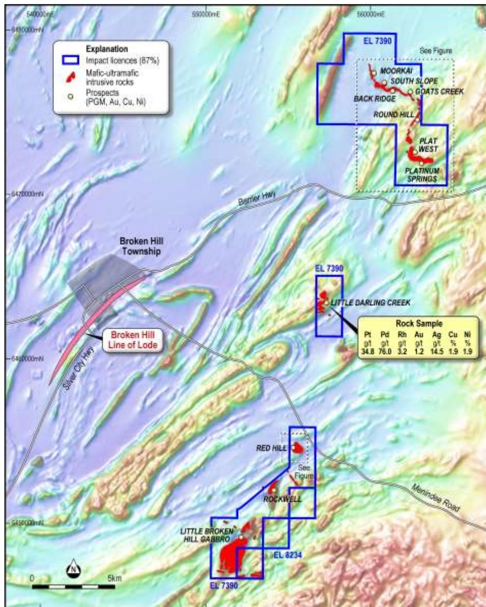
**Figure 2.** Image of airborne magnetic data showing the host rocks to PGM mineralisation (Red)
