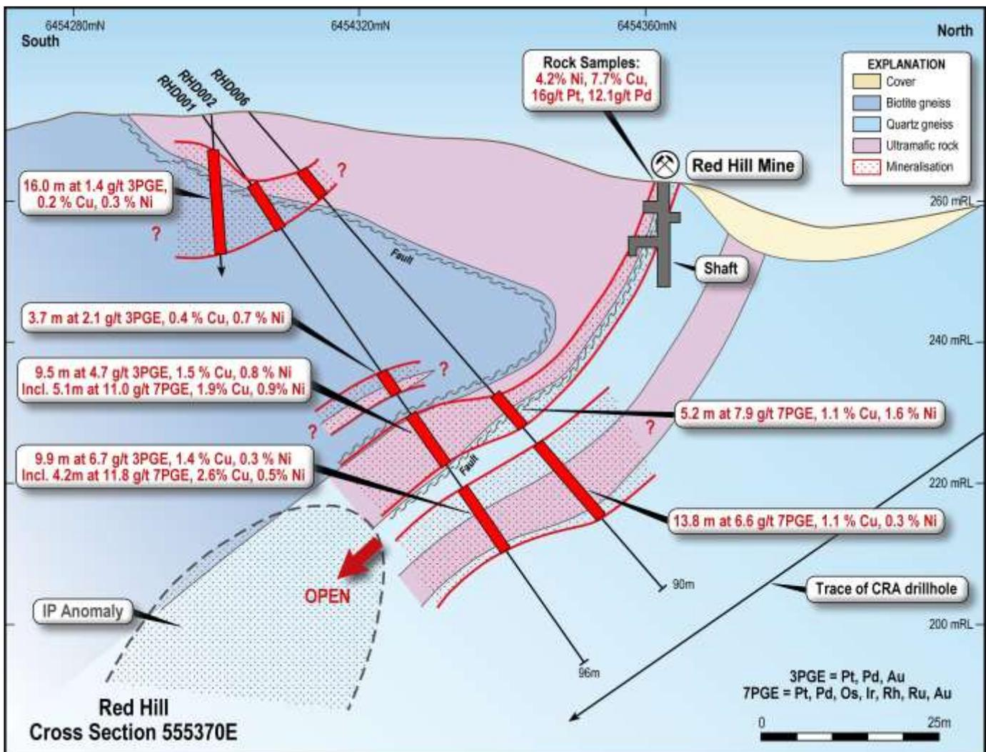
Figure 3. Cross section at the Red Hill Mine (see Figure 3 for location)
