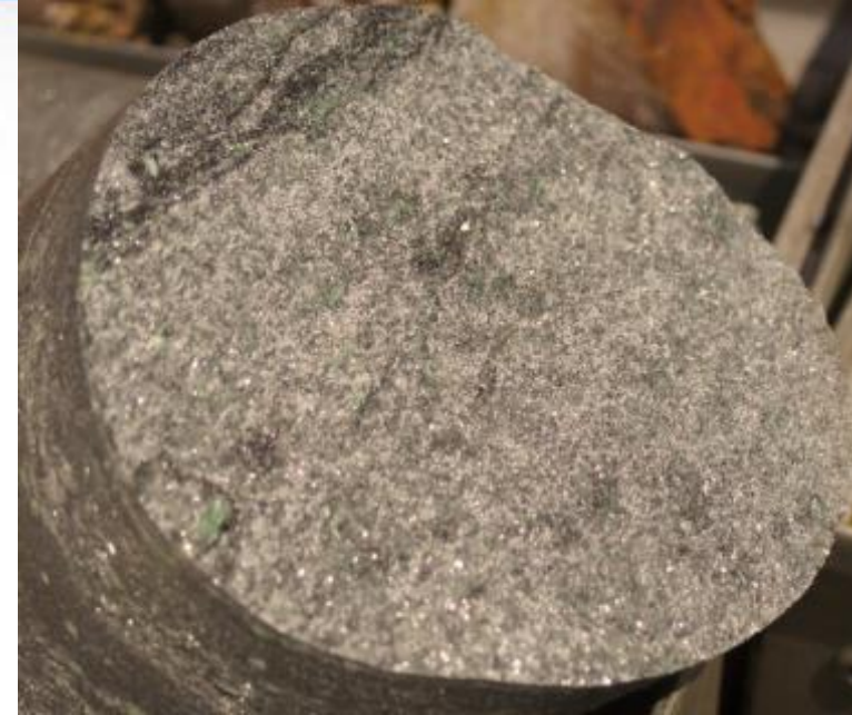
Diamond drill core from Nicanda Hill prospect on License 5966 showing graphite and vanadium
