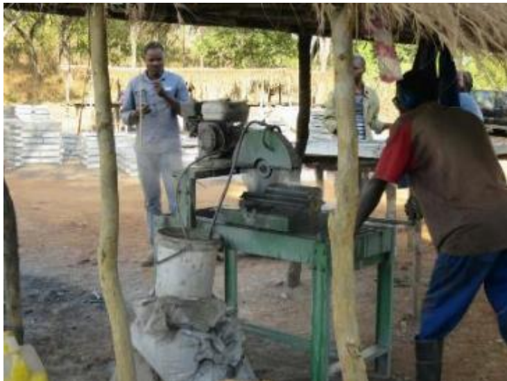
Triton geologists and field hands cutting diamond core at Nicanda Hill prospect (Source: www.thebutterflytree.org.uk )
