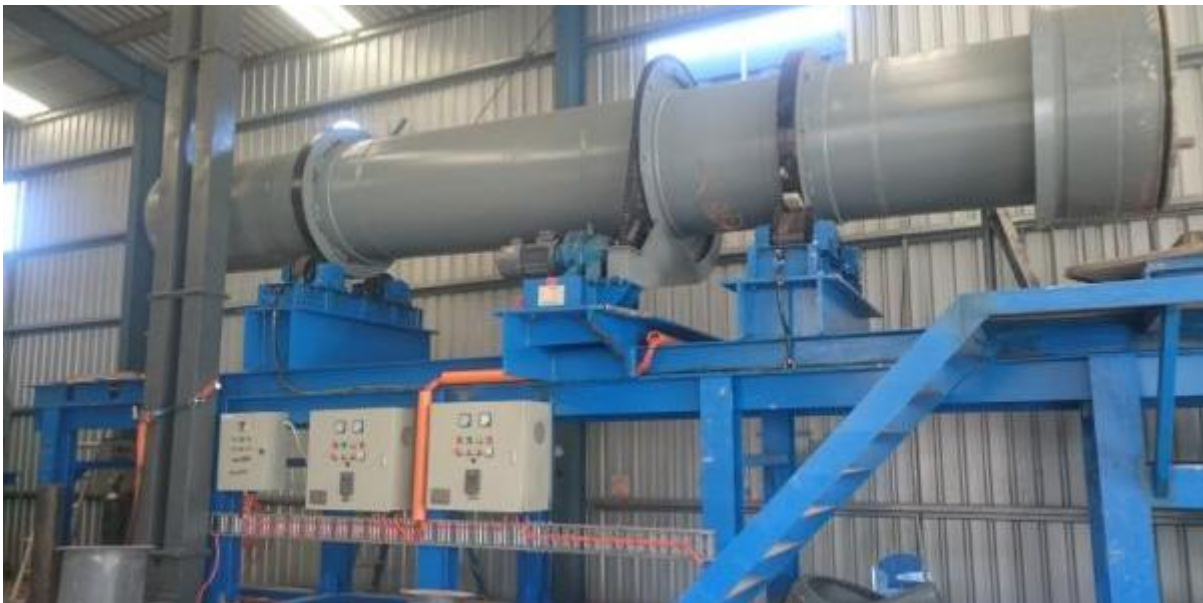
Image 1: Rotary Kiln and Rotary Cooler controls fitted.
