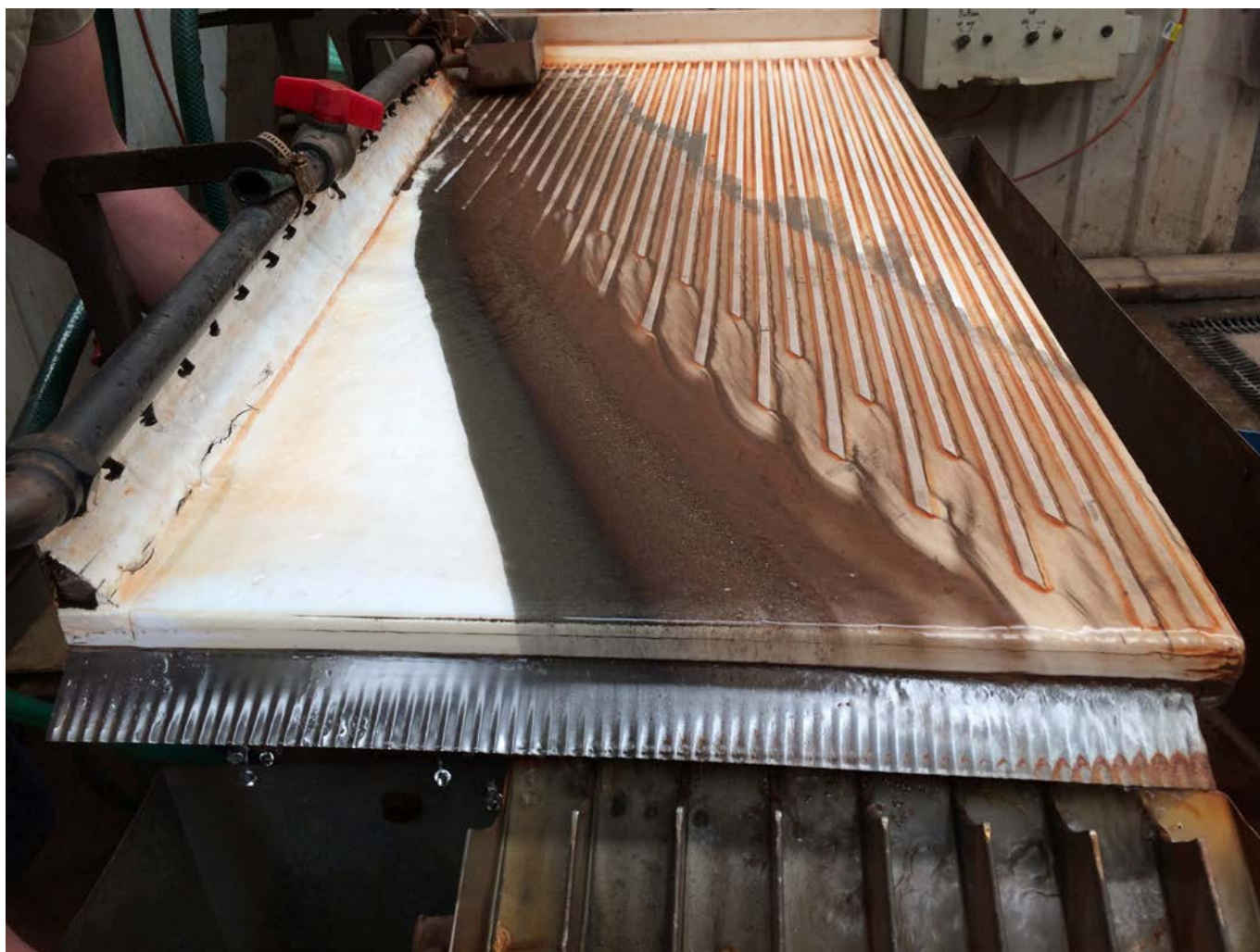
Plate 1 – Wet Table processing tailings from Composite Sample 1 with apparent sulphides (grey/black) separation.
