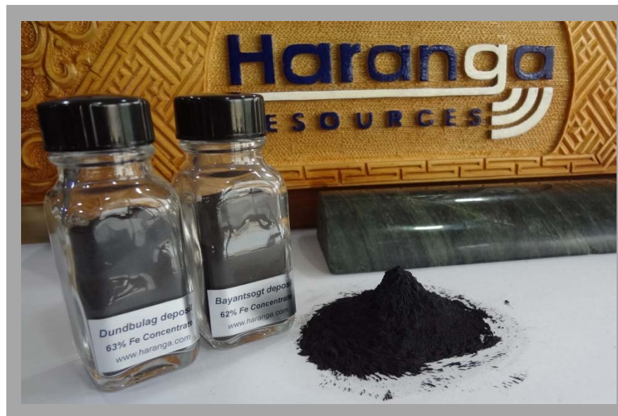
Dundbulag and Bayantsogt deposit iron ore concentrates extracted from metallurgical tests
