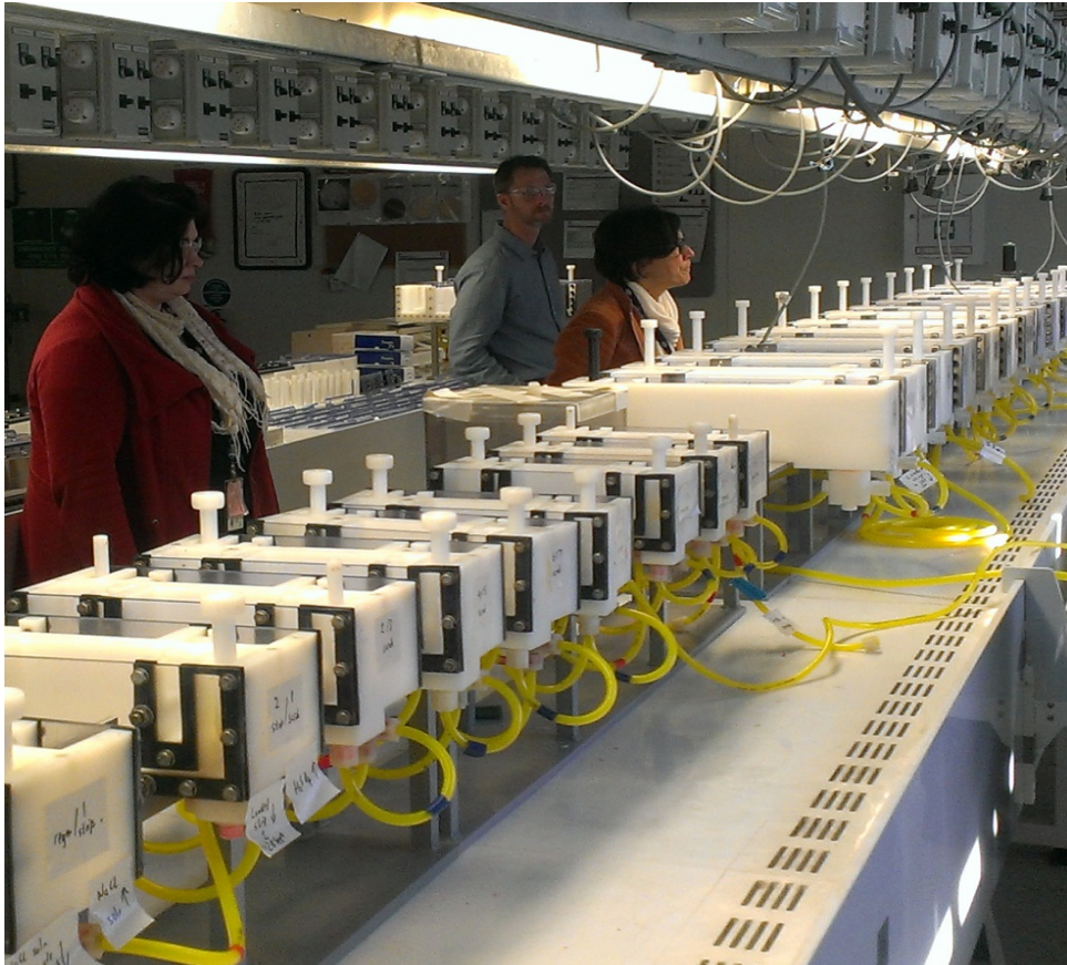
Alkane hafnium solvent extraction trials at ANSTO
