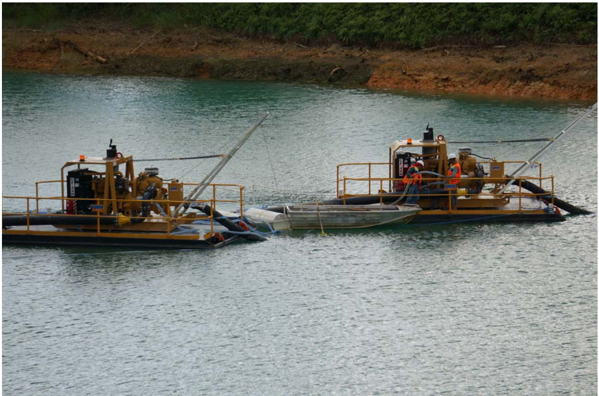
Figure 5. Dewatering activities at the Belinau open pit
