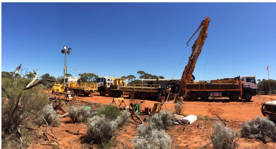
Figure 3: DDH1 high powered Sandvick multipurpose RC/Diamond truck mounted rig
