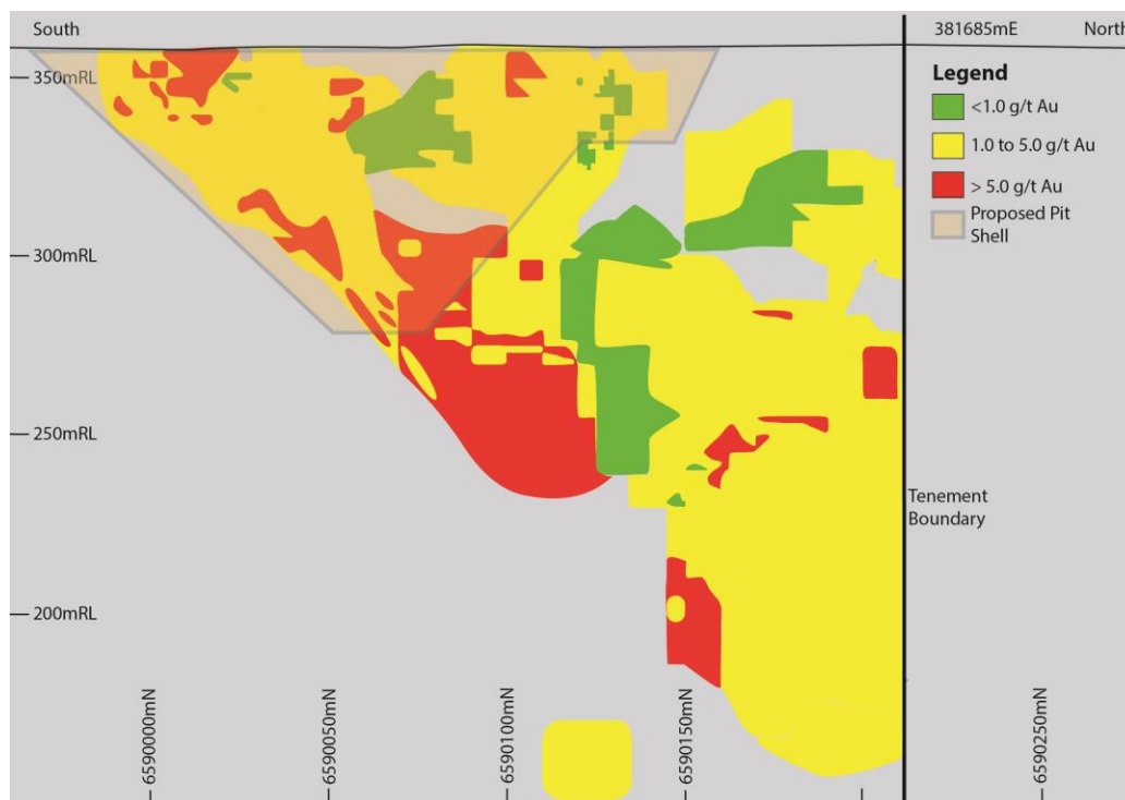
Figure 3: Long Section (looking west) of Cannon Resource by Au Grade on Section 381685mE with pit shell
