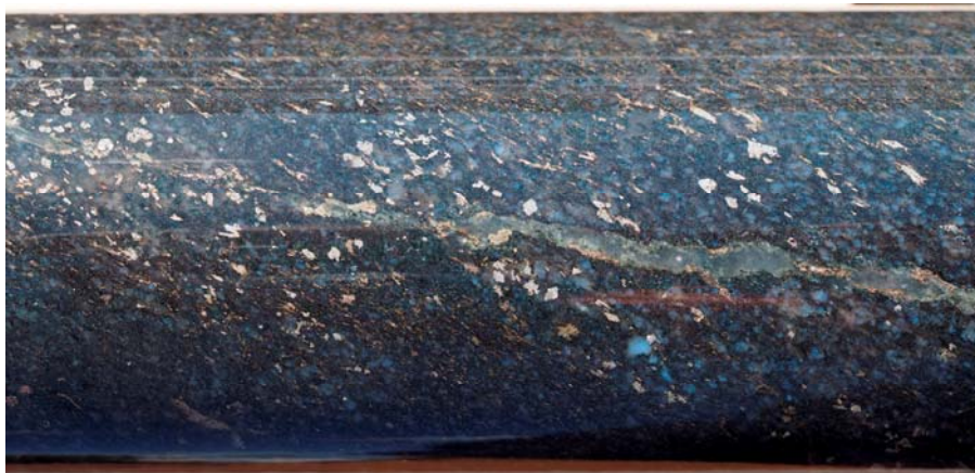
Figure 4: Drill core from diamond hole 15SYDD0001, 261 metres: strongly altered and sheared dolerite from within the main altered structure displaying remnant blue-quartz within an alteration assemblage of biotite-carbonate-albite-pyrrhotite-arsenopyrite.
