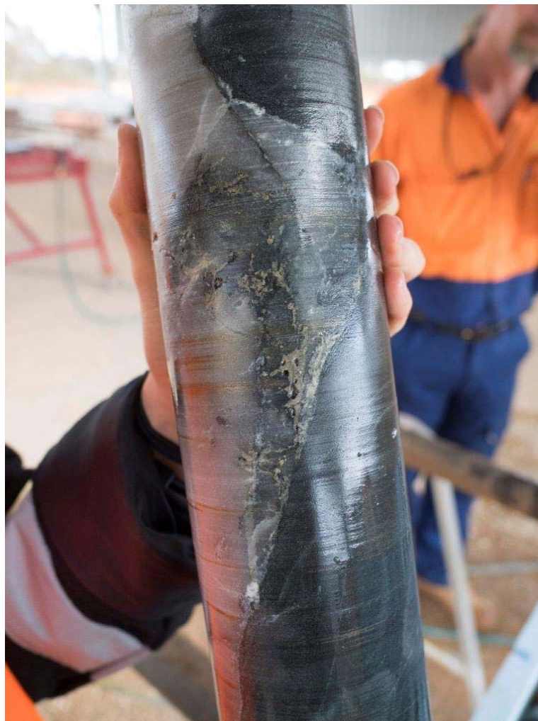
Figure 3: Drill core from hole 15EIS001 which is in progress. Close view of quartz vein with fracture fill sulphides (pyrite-pyrrhotite) in dolerite host.
