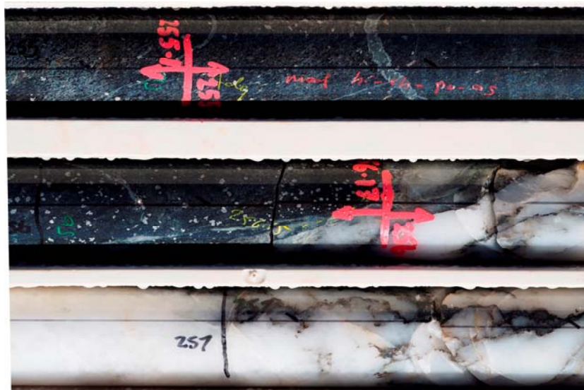
Figure 5: Drill core from diamond hole 15SYDD0001, 255-257 metres: margin of a quartz vein located in central part of the main shear zone with strong biotite-carbonate-albite-pyrrhotite-arsenopyrite alteration within coarse quartz-rich dolerite.
