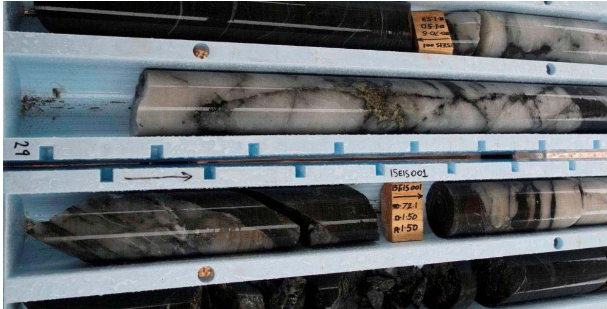
Figure 2: Drill core from hole 15EIS001 (70 to 72 metres) which is in progress. Fractured quartz veins with sulphide-biotite alteration hosted in equigranular dolerite.
