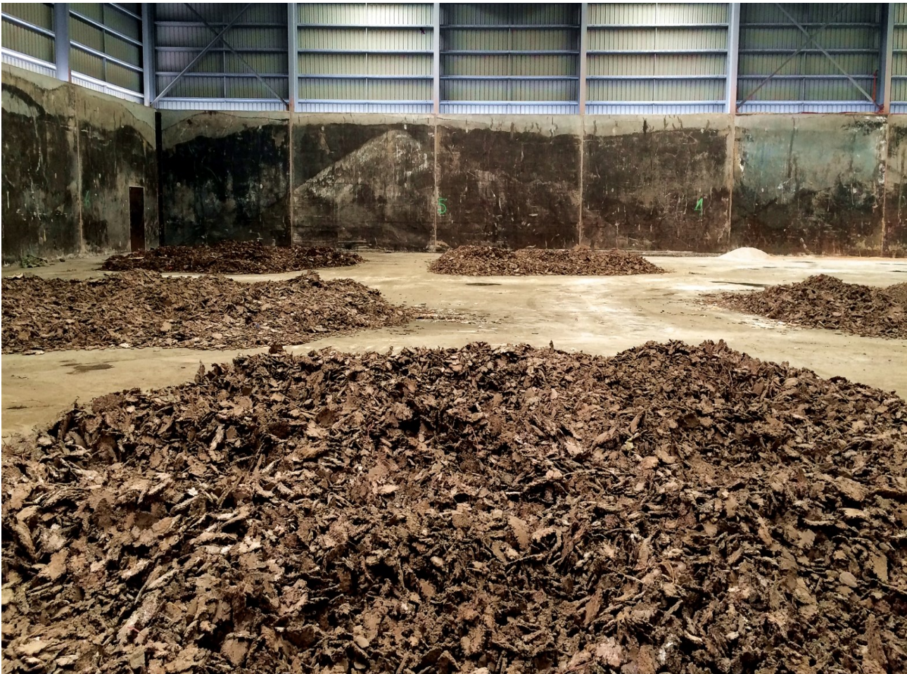
Figure 1: Part of a consignment of oversize native copper metal concentrate ~95% Cu, tipped into 23 tonne piles (half-container for each pile) at the Port of Townsville, for the purpose of umpire sampling and customs audit.
