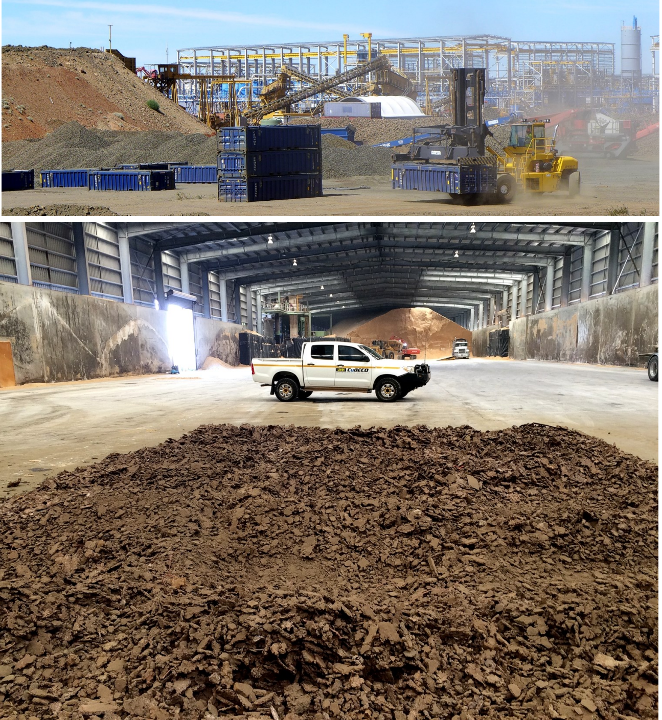
Figure 3: Containers being loaded at Rocklands (top image); and native copper in storage at the Port of Townsville, re-combined for loading back into containers after being selectively tipped out for umpire sampling and customs audit.
