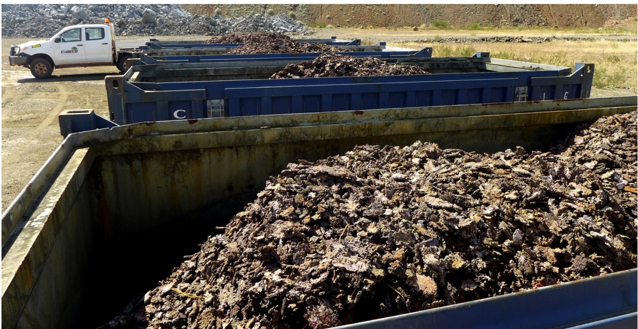
Figure 2: Simple crushing and screening of coarse native copper ore is generating an extremely high-grade native copper metal product (~95% copper) suitable for interim sales and early cash-flow.
