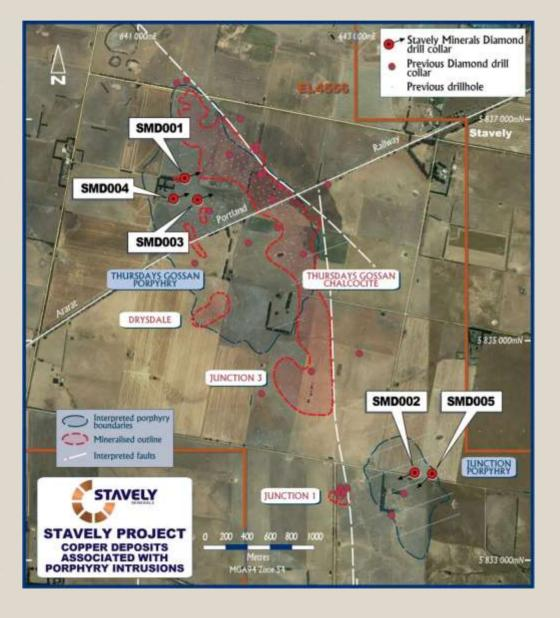
Stavely Minerals drilled 3 deep diamond drill holes (between 532m to 640m deep) into an induced polarisation (IP) chargeability anomaly
