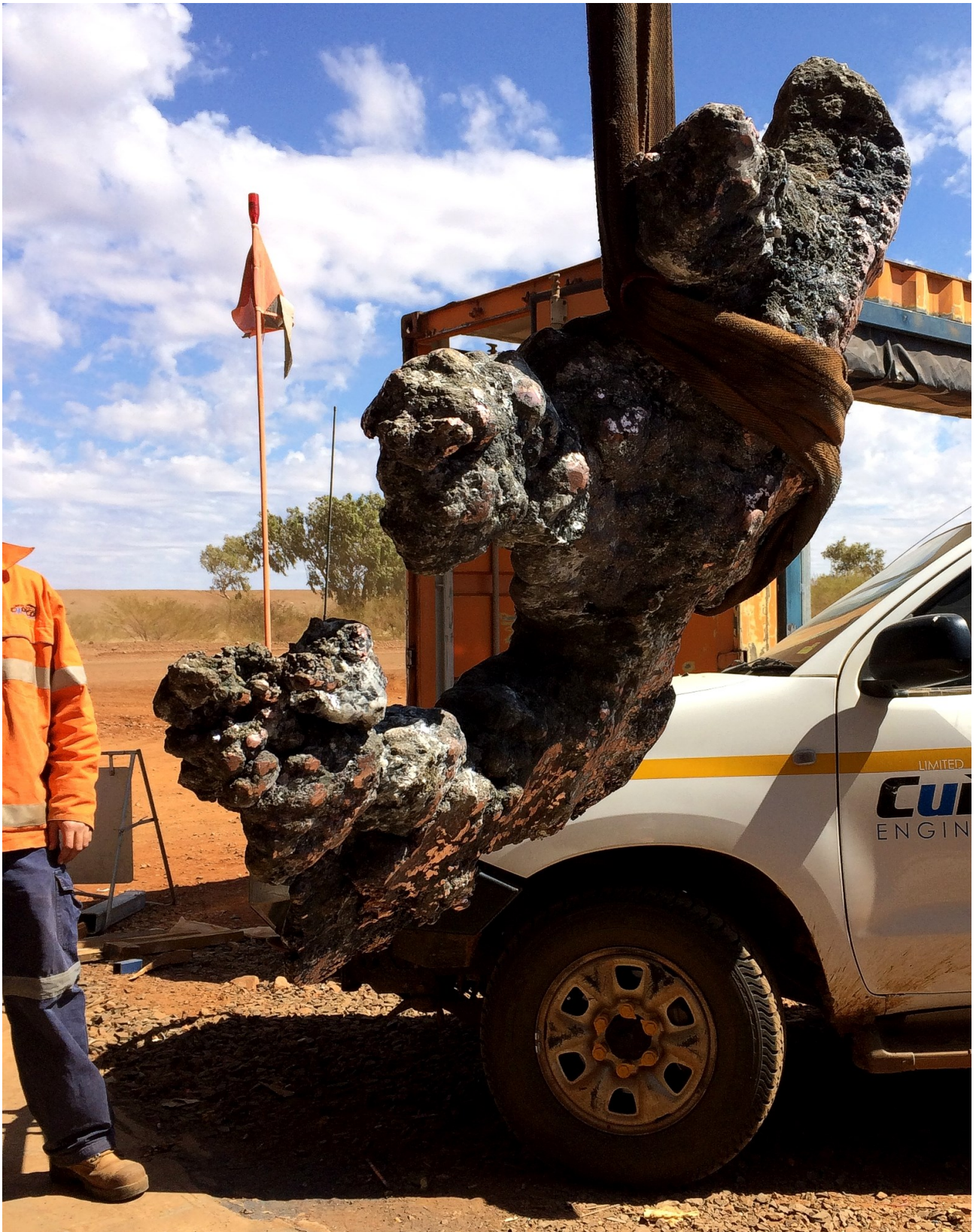
Figure 2: Example of native copper masses being recovered from the pit - not intersected by resource drilling.
