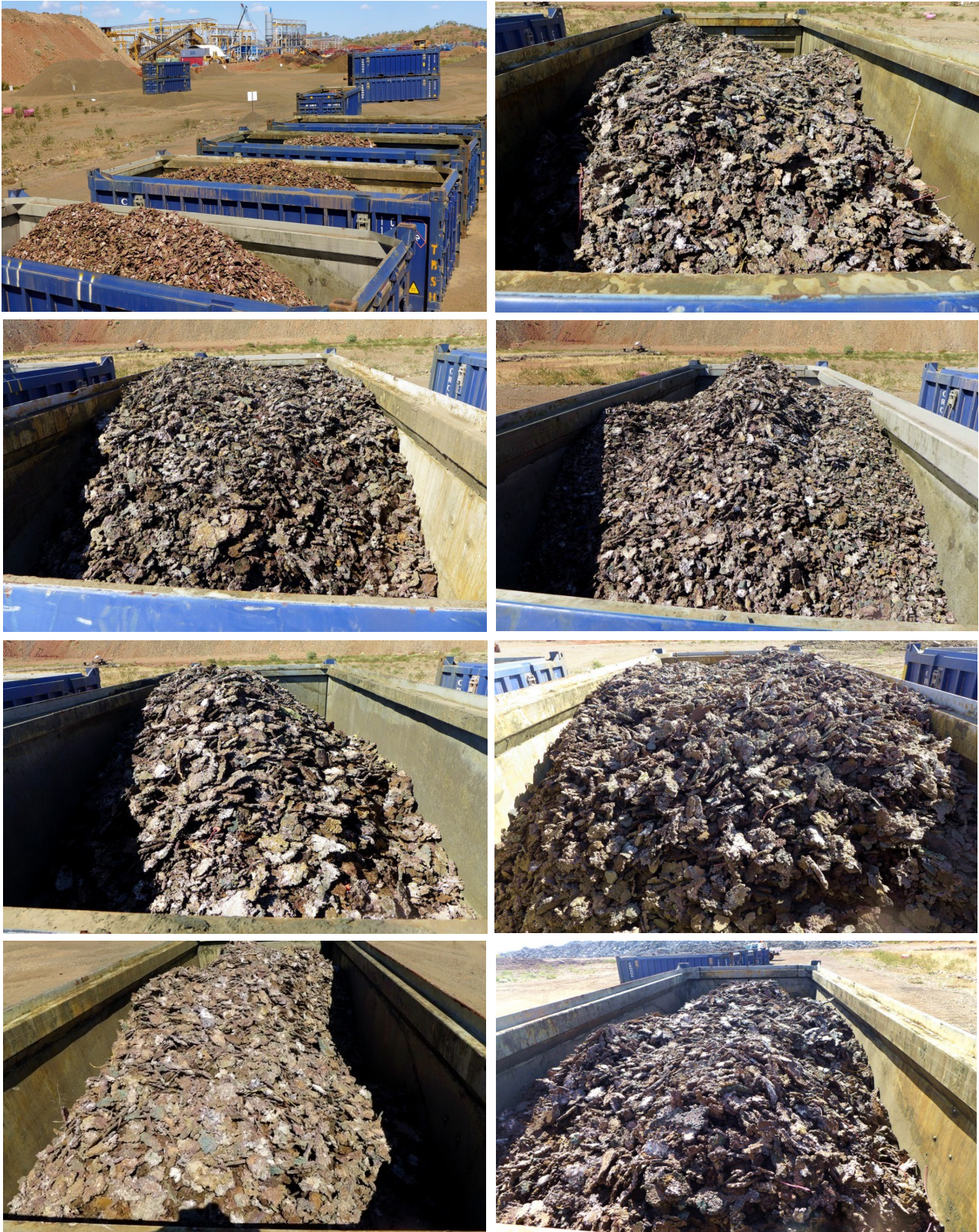
Figure 12: Coarse native copper circuit product averaging ~95% copper metal in concentrate. The purpose of this circuit is to remove oversize native copper (+40mm) prior to commencement of processing in main mineral processing plant under construction.
