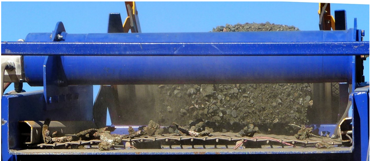
Figure 8: Scalping (recovery) of coarse native copper by simple crushing and screening. The native copper is flattened during cone-crushing whereas the rock breaks into smaller pieces, facilitating easy removal via appropriate screen sizing.
