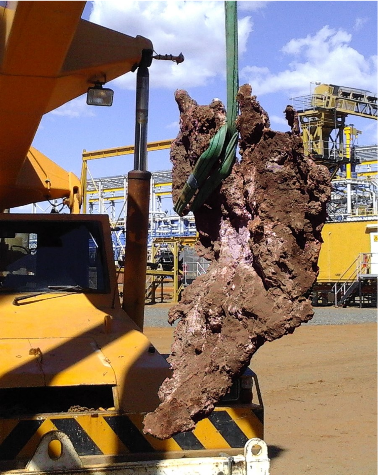
Figure 4: Part of a much larger native copper nugget retrieved from the jaw crusher - not intersected by resource drilling.
