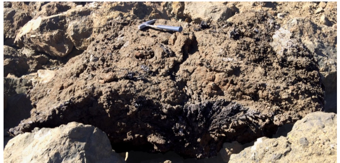
Figure 5: Example of native copper masses being recovered from the pit - not intersected by resource drilling.
