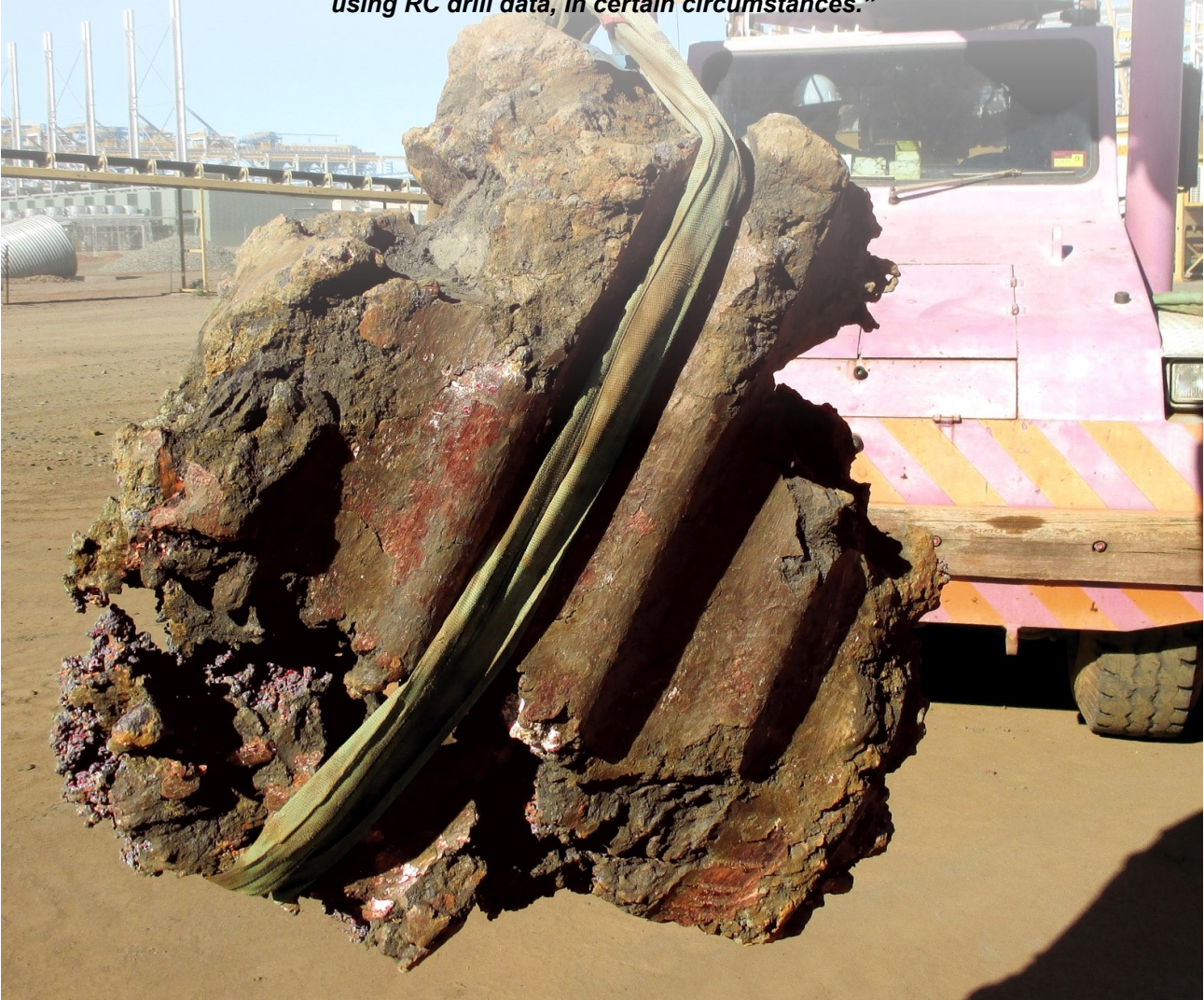
Figure 1: Example of native copper masses being recovered from the pit - not intersected by resource drilling.
