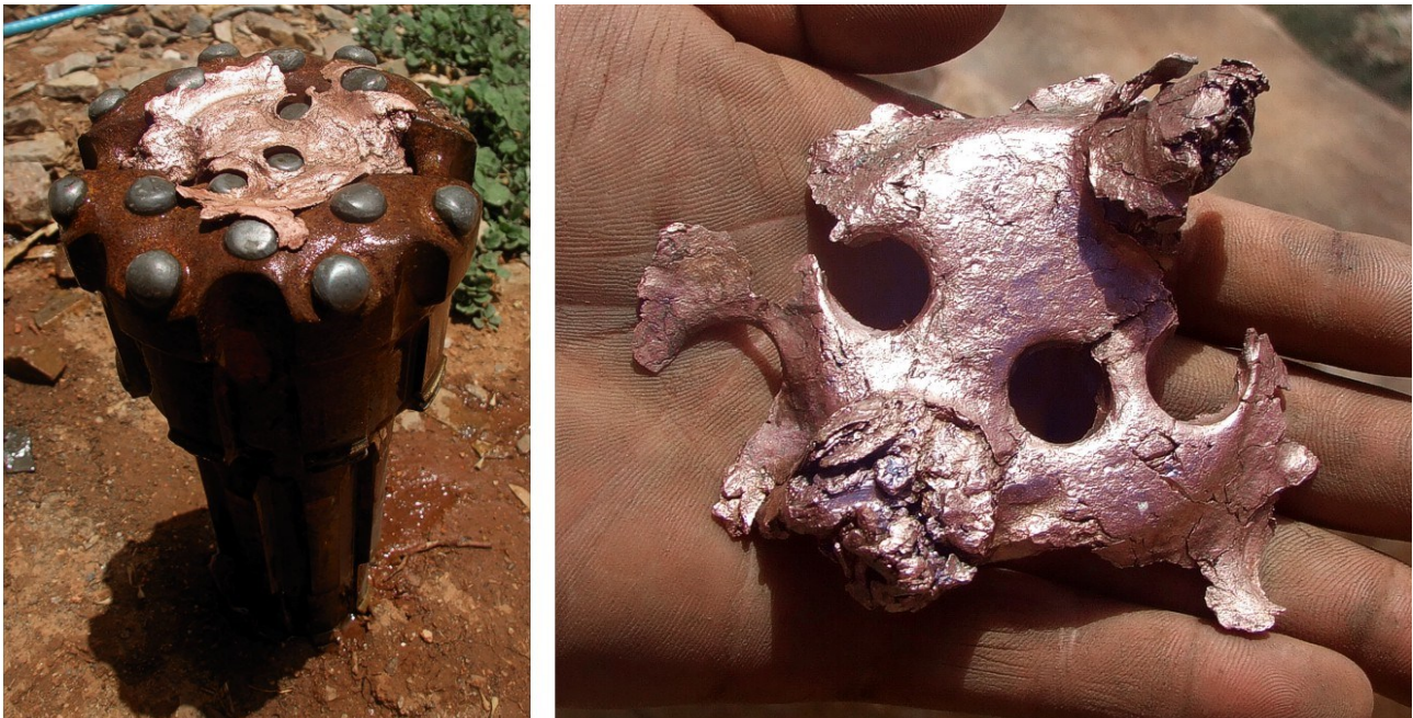
Figure 10: Example of large native copper nugget, possibly encountered in soft clay or friable oxide material and unable to return up the small (20mm) sample return holes at the end of the RC bit. Left; the remaining middle section appears to have been "stamped" out of a larger solid copper nugget that has been flattened, then cut through by the bit and right; underside of the copper "stamp" showing how the metal was pushed into the two sample return holes (top right & bottom left) and was unable to return to surface.
