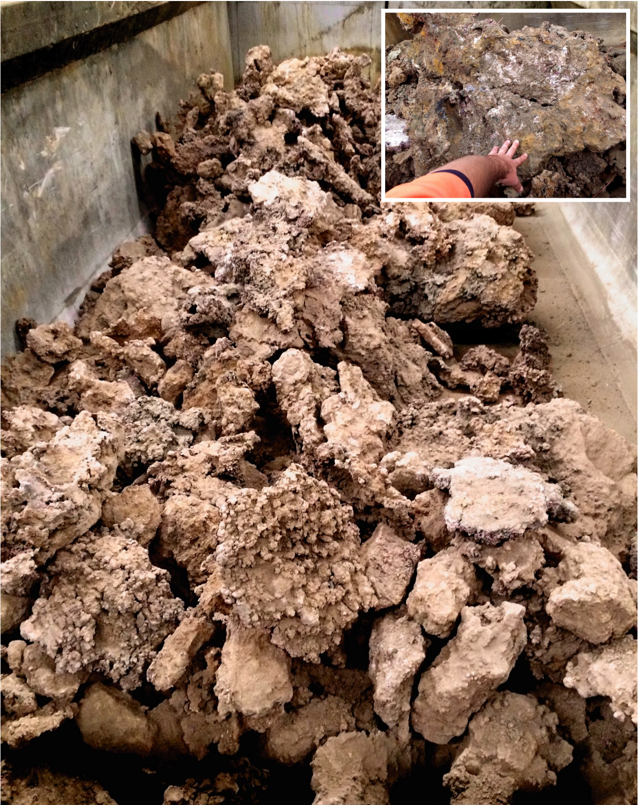
Figure 14: Oversize coarse native copper is loaded into containers as it is scalped during crushing. The majority of native copper at Rocklands is -40mm fraction size.
