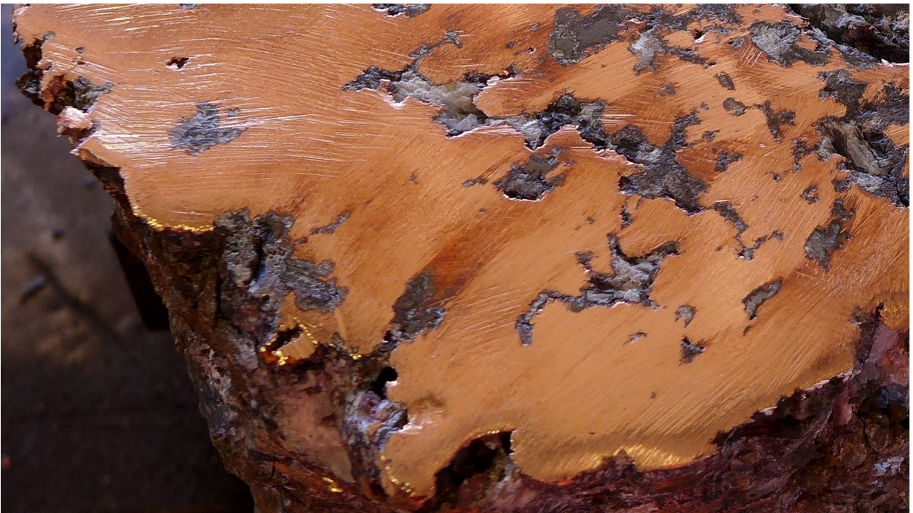
Figure 11: Large nugget cut with diamond saw revealing the near solid nature of the agglomerates - this sample estimated at 95% Cu by weight.
