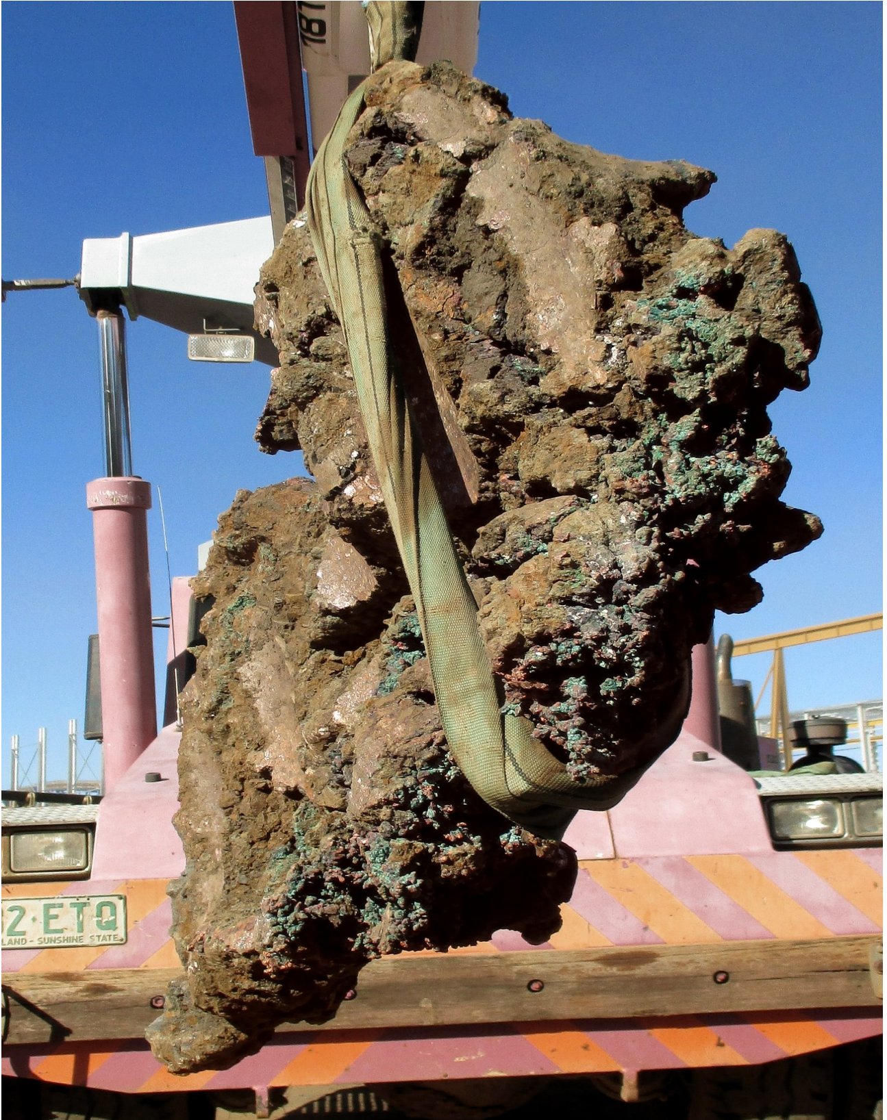
Figure 3: Example of native copper masses being recovered from the pit - not intersected by resource drilling.
