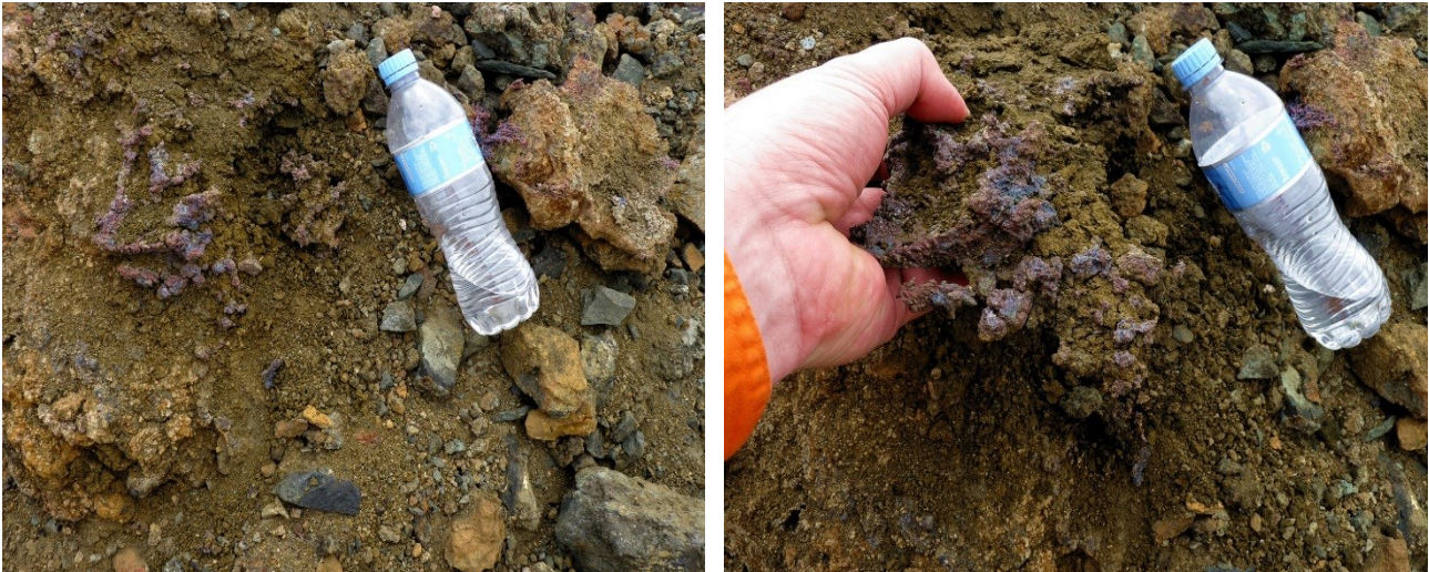
Figure 9: Example of high-grade native copper ore in soft friable matrix (dry green clays) in Las Minerale (LM1) pit, highlighting ease of pulling native copper nuggets by hand from the ore/rock-face. It is postulated drilling in soft matrix is unlikely to recover similar coarse native copper nuggets, which are likely to be pushed into the surrounding soft matrix rather than return to surface through the RC bit's 20mm wide sample return holes.
