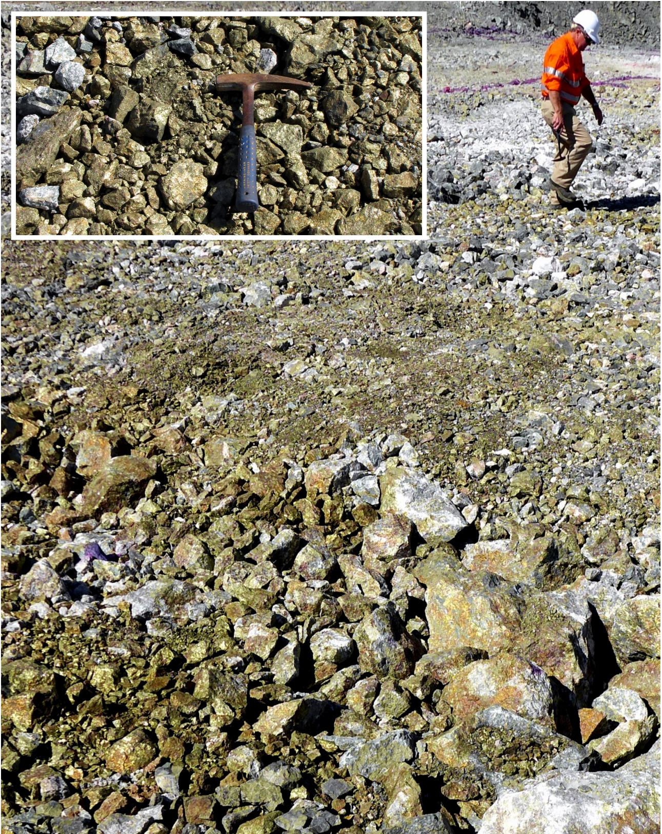
Figure 15: LM2 Pit floor at RL195 - high-grade primary copper ore (chalcopyrite) including massive, semi-massive, breccia, fracture infill, and disseminated, strewn across the pit floor, likely to have facilitated the formation of bonanza zones of coarse native copper.
