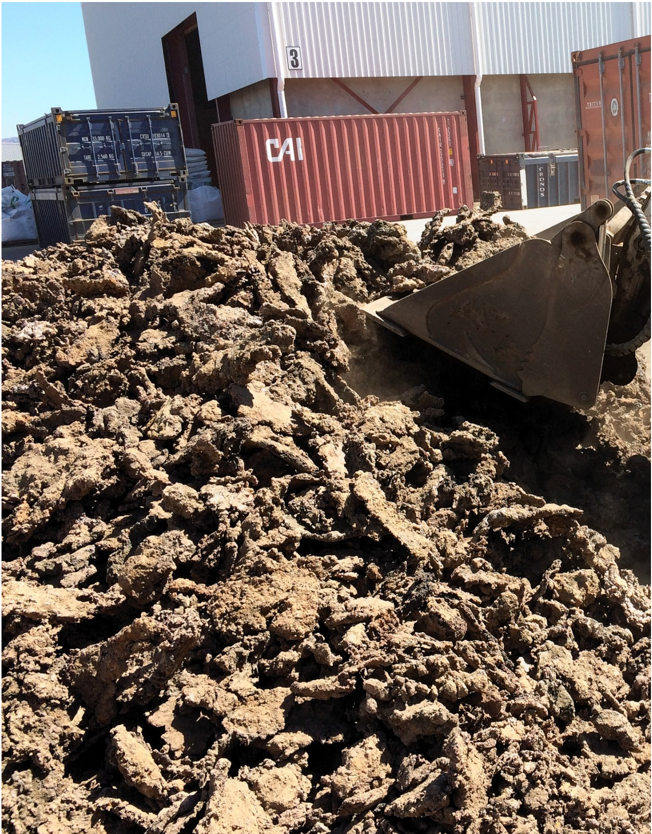
Figure 13: Coarse native copper product averaging ~95% copper metal in concentrate at the Port of Townsville
