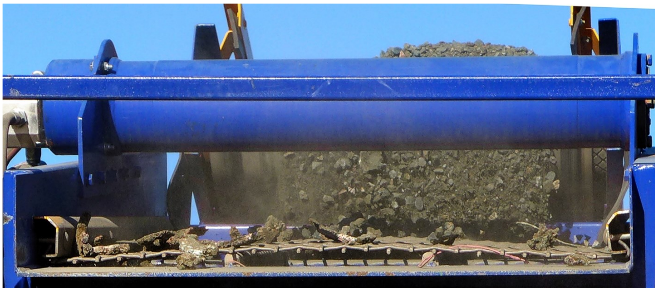
Figure 8: Scalping (recovery) of coarse native copper by simple crushing and screening. The native copper is flattened during cone-crushing whereas the rock breaks into smaller pieces, facilitating easy removal via appropriate screen sizing.
