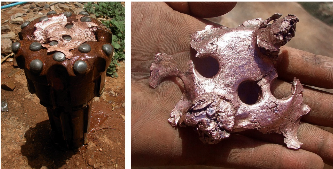
Figure 10: Example of large native copper nugget, possibly encountered in soft clay or friable oxide material and unable to return up the small (20mm) sample return holes at the end of the RC bit. Left; the remaining middle section appears to have been "stamped" out of a larger solid copper nugget that has been flattened, then cut through by the bit and right; underside of the copper "stamp" showing how the metal was pushed into the two sample return holes (top right & bottom left) and was unable to return to surface.
