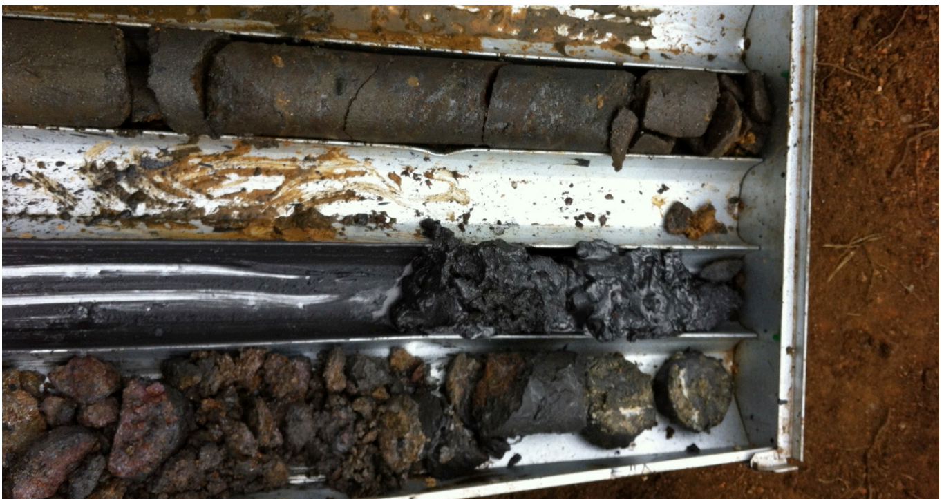
Photos 5,6. Diamond drill at DD06, Epanko northeast. Core from DD06. Graphite intersection from 45m to 73m.
