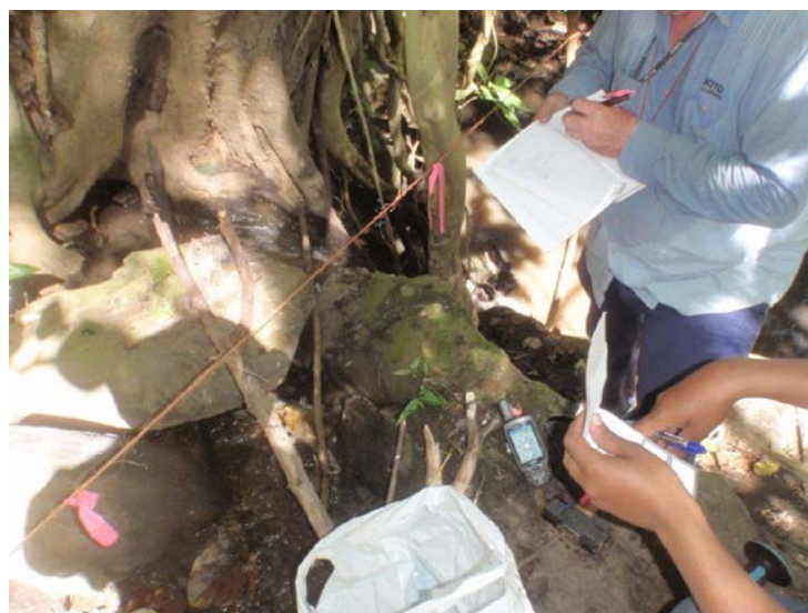
Photo 9. Graphite mineralisation being mapped and sampled at 1m intervals along creek exposure. Five outcrop samples taken along this creek in 2014 averaged 10.06% TGC. The current sample programme will provide much more detail about the geology, width and grade of this graphite mineralised zone
