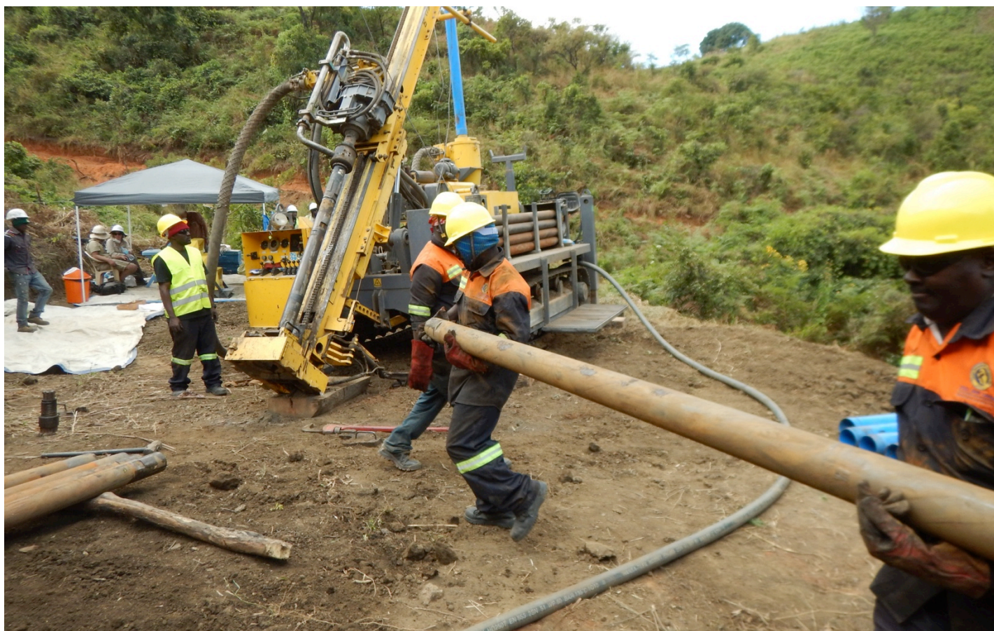
Photos 2, 3. RC rig drilling at Epanko north and logging RC samples.
