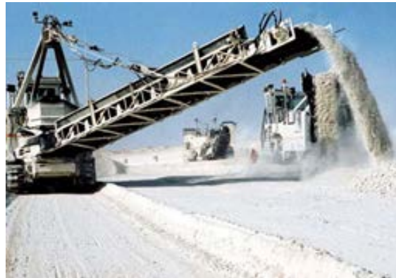
Wirtgen Surface Miner Cutting Salt
