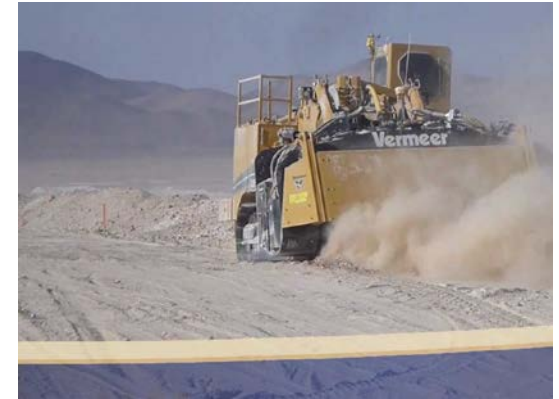
Salt extraction using surface miners
