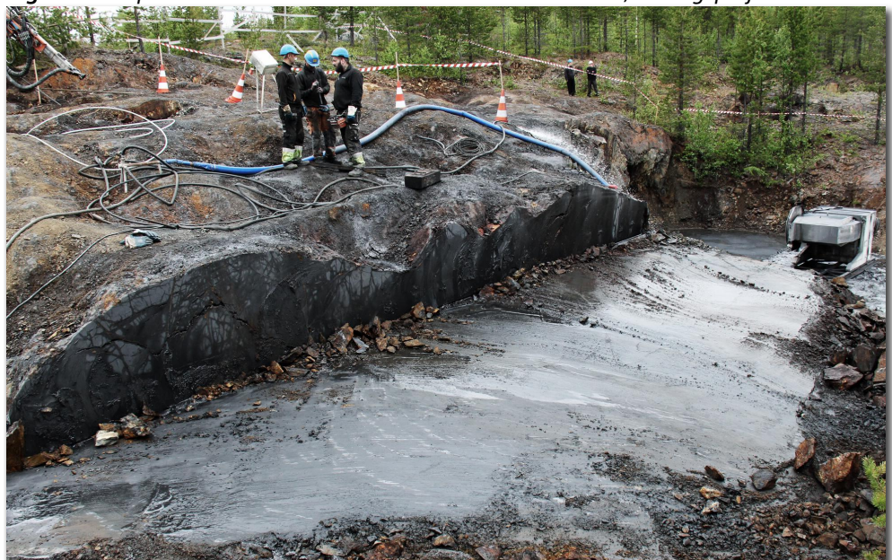
Figure 1 - Preparation of first trial mine ore bench at Nunasvaara, Vittangi project.
