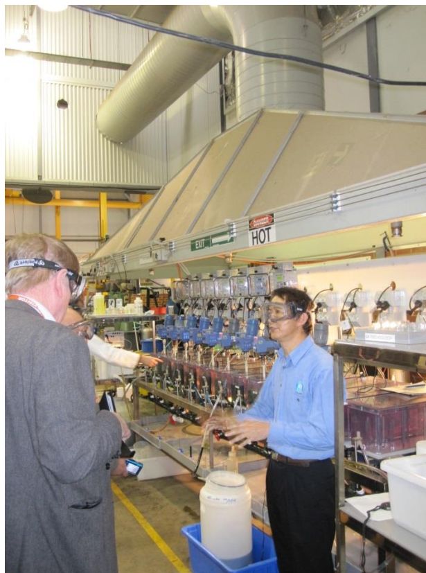
Dr Wensheng Zhang, (CSIRO) explaining the operation of the industry standard solvent extraction circuit.
