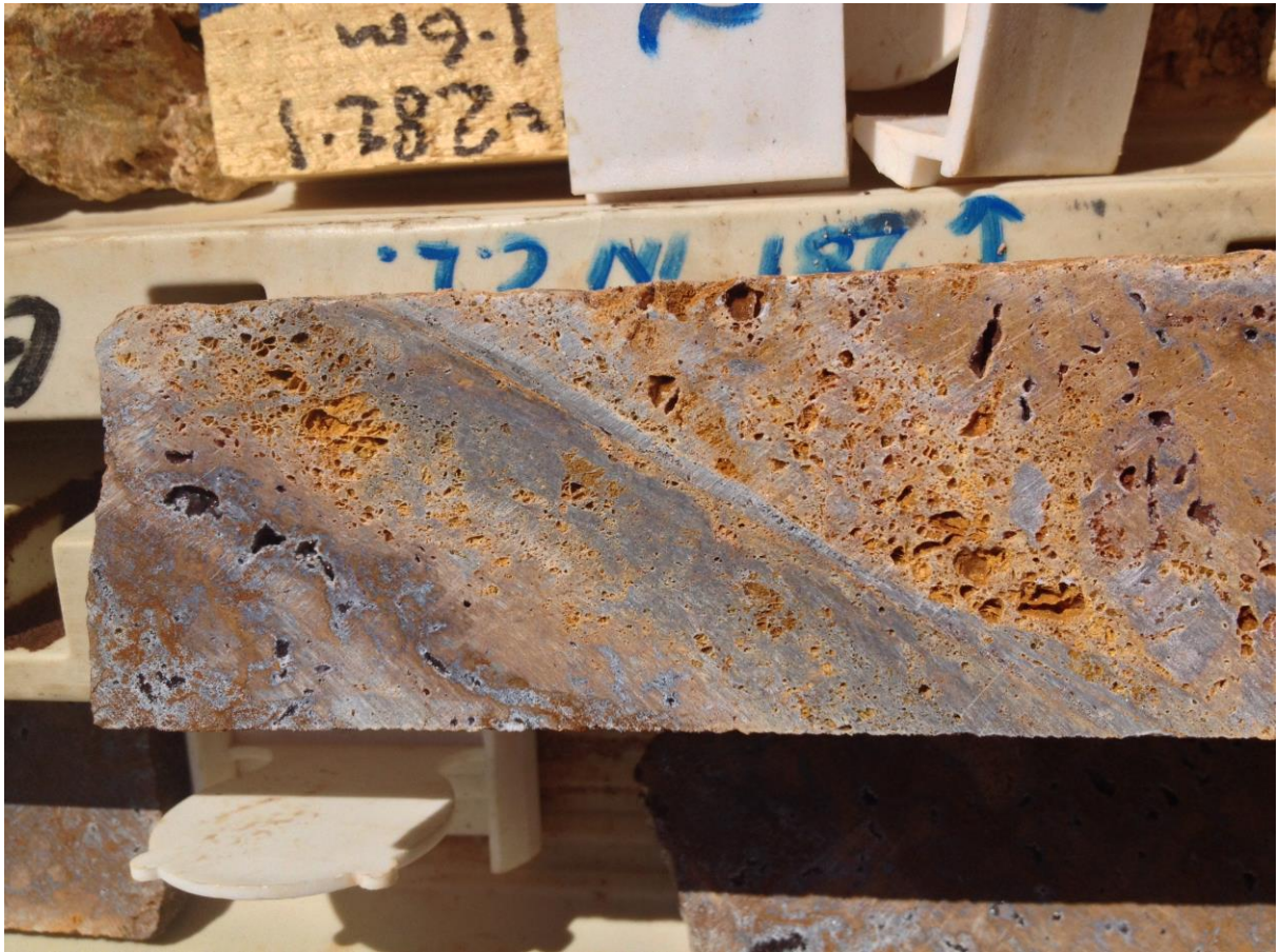
Photo: Gossan sample from 281 metres in drillhole EPT2201
