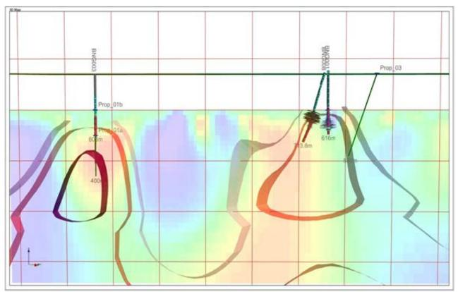
Figure: Bungalien Project. The Bronzewing Bore Prospect and The Brothers' Prospect. A section along 207° looking WNW through the 3D magnetic inversion model (shells) and voxel gravity model (background image). Drill traces for existing holes BNG001, 8 and 3 (including the extension now in progress) shown. Drill-lithology modulated in thickness for magnetic susceptibility.
