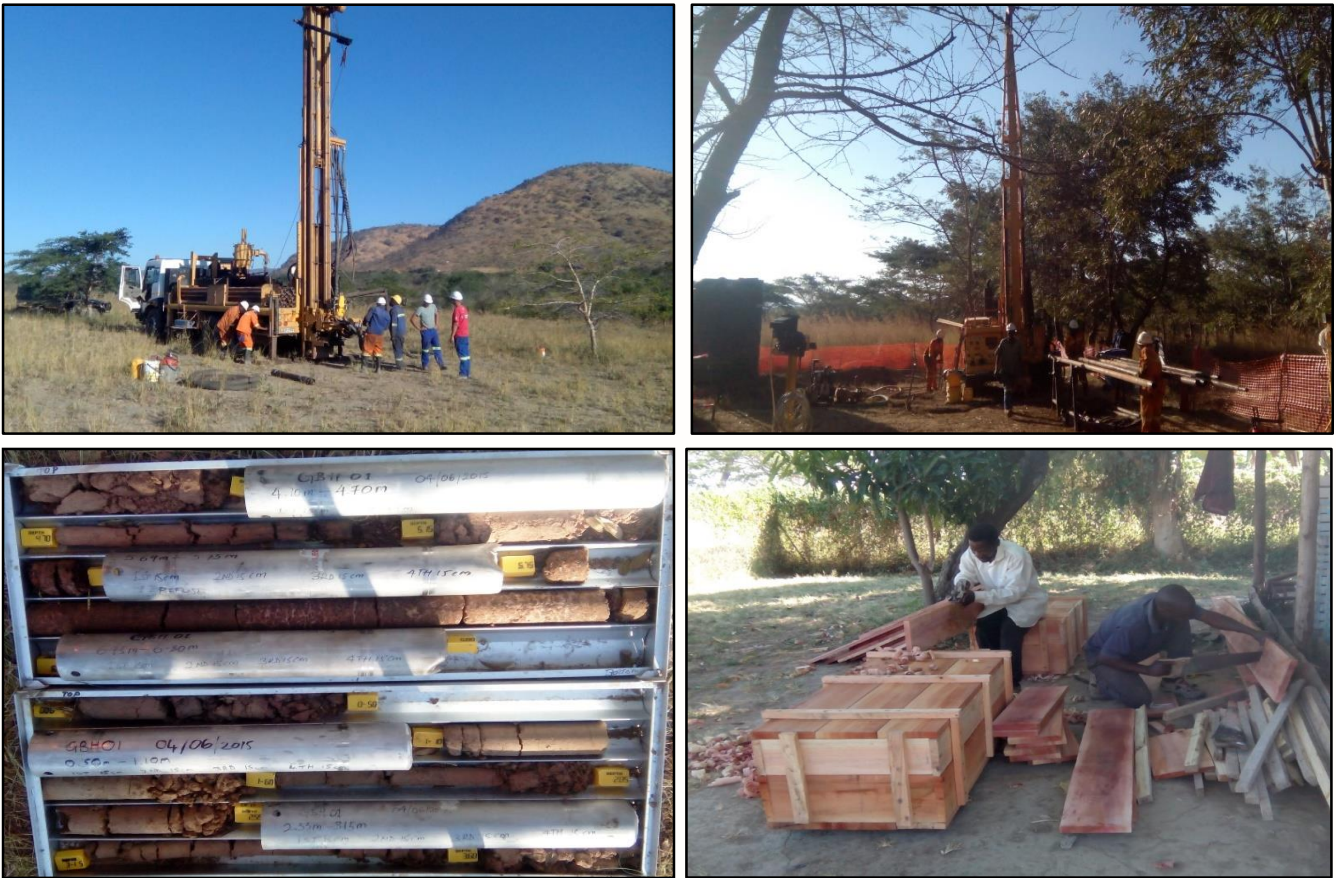
Figure 3: Showing hydrological drilling near the base of Panda Hill (top left), drilling for geotechnical samples in the TSF region (top right), geotechnical core samples (bottom left) and carpenters preparing boxes to transport the samples to South Africa (bottom right).
