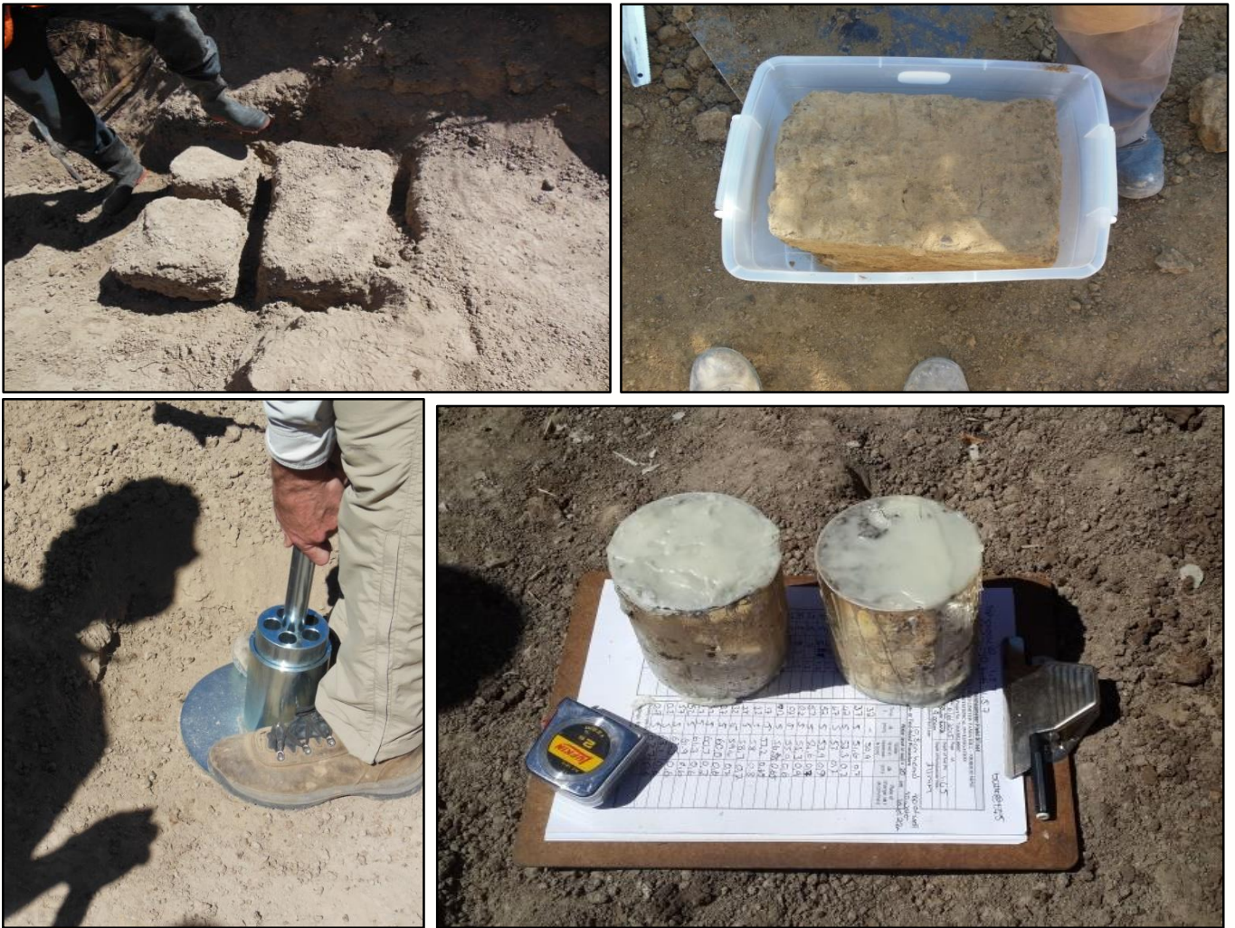
Figure 4: Showing in situ geotechnical block samples being collected (top); Shelby Tube samples being taken from bottom of pits (bottom). These samples will be used to assist in gauging the ground conditions for the Tailings Storage Facility.
