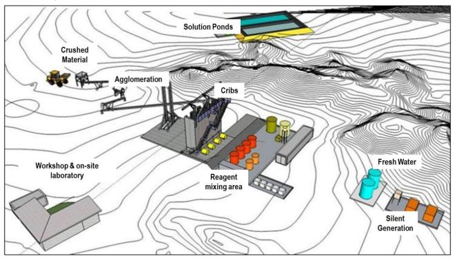
The photograph below shows the plant site from the north east. The plant is self-sufficient with respect to electricity and operates on a continuous cycle. The cribs are able to be operated in open (i.e. individually) or closed loop (i.e. in series) circuit. The latter allows simulation of the full scale operation of heap leach pads.
