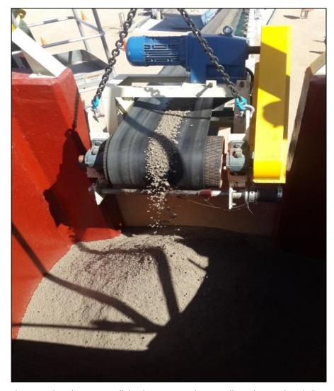
The agglomerated ore used in the two parallel columns per crib was collected on an hourly basis from the conveyor stacking the crib concerned and then loaded into the columns using a sample bag. Care was taken to maintain the one meter drop height whilst loading the columns.
