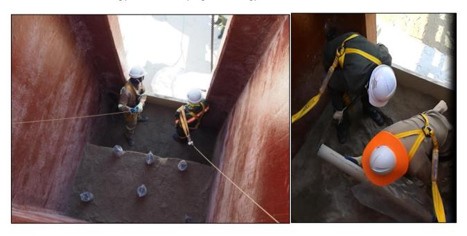
Heap stability and the integrity of the agglomerates were clearly evident during unloading process. As expected slight segregation of ore due to the stacking was observed at each meter segment, with the finer content located in the centre as shown in the photograph below. However no percolation issues were observed.
