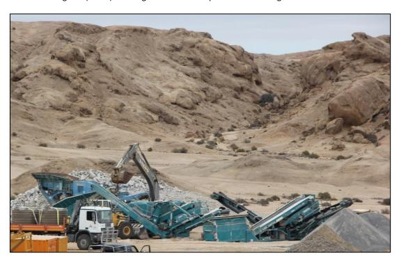
Over and above generating material similar to that specified in the DFS, two other samples were generated to enable future value engineering studies. These were coarser HPGR and conventional crushed material. Waste material (Gneiss rock) to be used for ore dilution purposes was crushed in a similar manner. The ore and waste stockpiles generated are shown in the photograph below.
