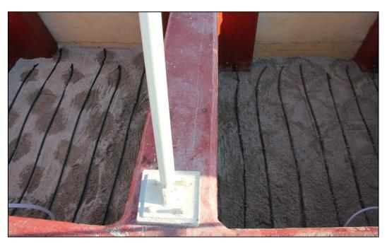
Leach irrigation was conducted for 20 days followed by a post leach drain of 2 days and then a rinse and post rinse phase of 3 days and 5 days respectively. A weak sulphuric acid solution (2 g/l) was used as rinse solution.
