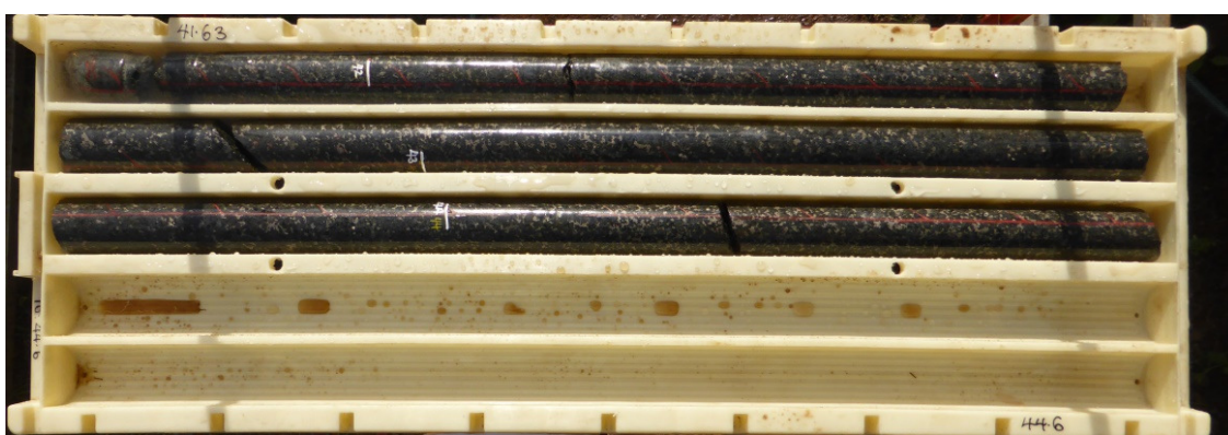
Figure 1 AKD009 41.6m to 44.6m coarse matrix textured sulphides
