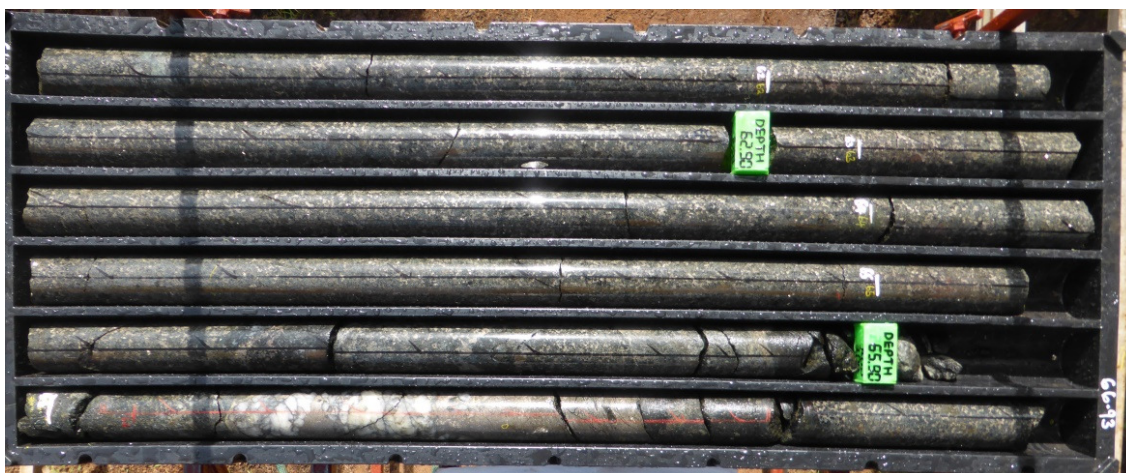
Figure 2 AKD009 61.3m to 66.1m coarse disseminated sulphide and 66.1m to 66.5m massive sulphide
