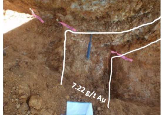
Figure 7 – Quartz vein 0.4m @ 7.22 g/t Au at Talang Toha
