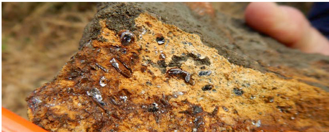
Photo 1. Coarse graphite flakes within outcrop at north Cascade. Graphite flakes are up to 7mm long.
