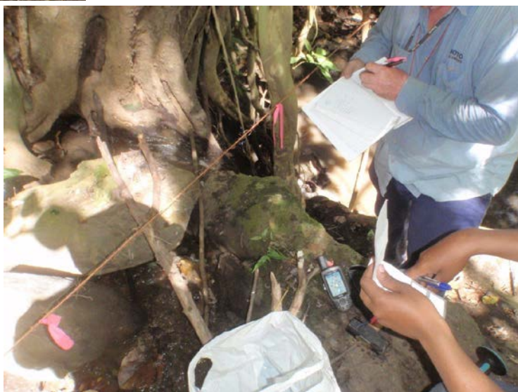
Photo 4. Graphite mineralisation mapped and sampled along creek exposure. Five outcrop samples taken along this creek in 2014 averaged 10.06% TGC. The current sample programme will provide much more detail about the geology, width and grade of this graphite mineralised zone
