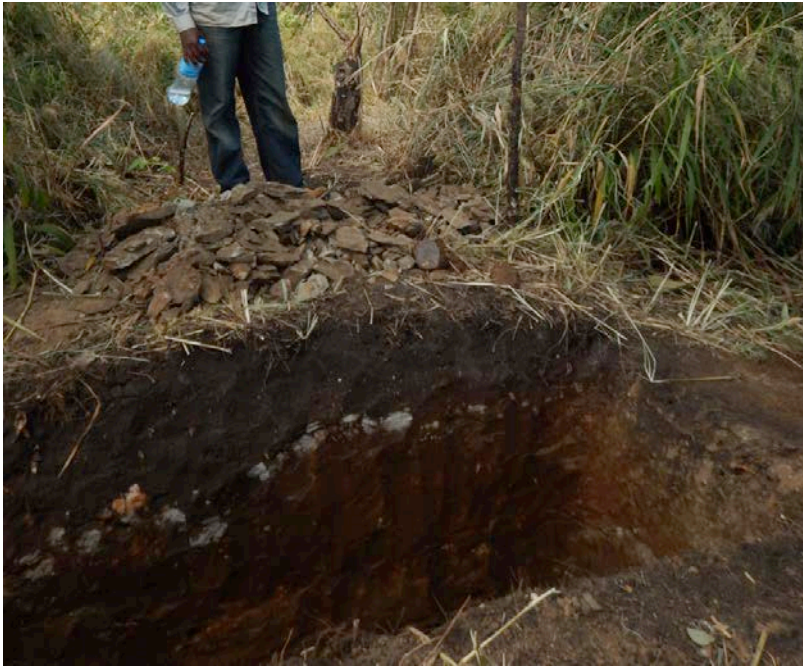
Photo 3. test pit at ridge top showing less than a metre of cover before exposing graphitic basement. Sample #088 returned 12.85% TGC
