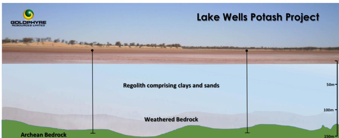
Figure 2: Lake Wells Potash Project, Schematic cross section with proposed drill hole trace demonstrating blade refusal penetration through regolith and deep palaeochannel section
