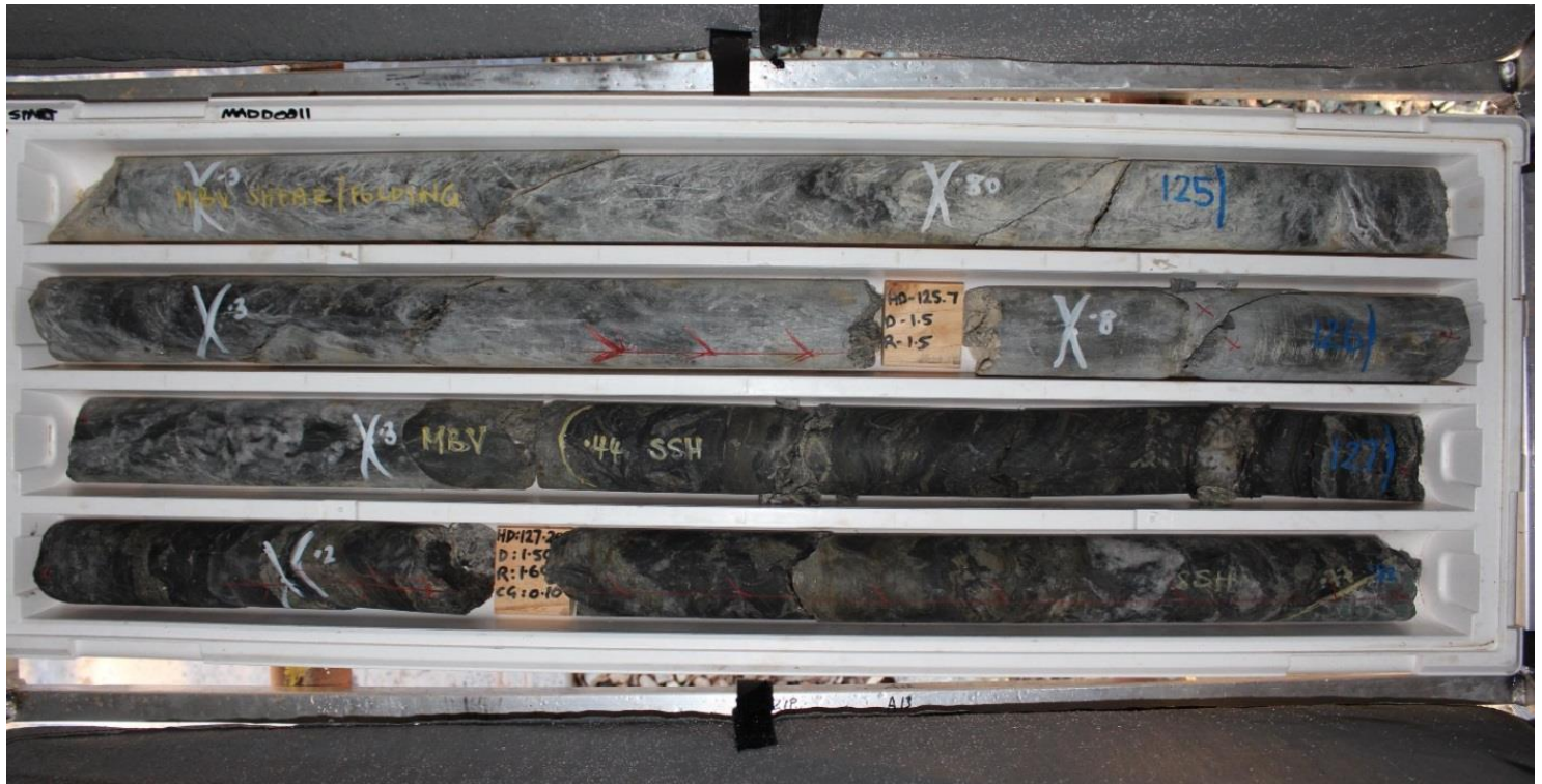
Photo 3: Strongly mineralised intersection in Matilda drill hole MADD0011 with visible sulphides, veining and shearing of basalt and shale host rocks (assays pending).
